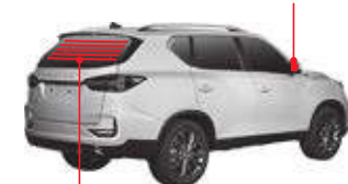
Rear window heater
