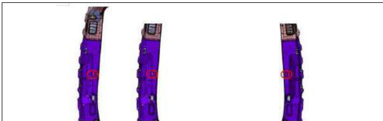
29 Tail lamp mounting hole (37-37, symmetry)
