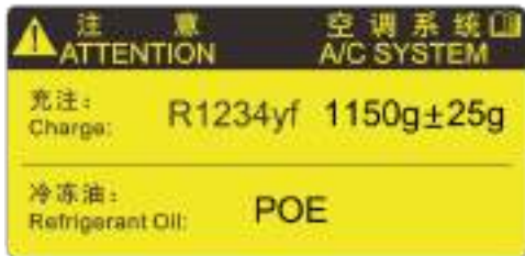
5. Air conditioning system label.
