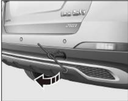
4. Tighten the towing ring securely with wheel dismantling wrench.
