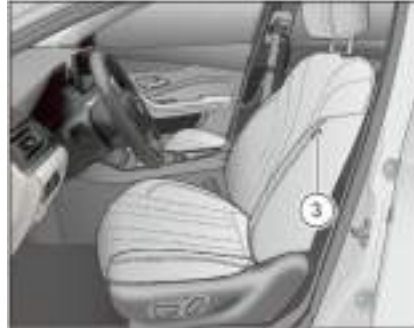
The side airbag ③ is located in the backrest lining of the front seat door side
