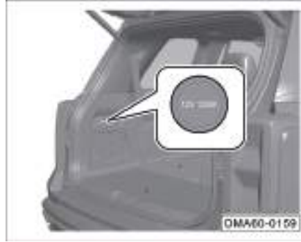
Trunk power outlet
