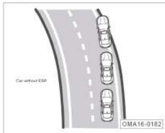
Vehicle not equipped with ESP sideslips and deviates from the normal route during driving.
