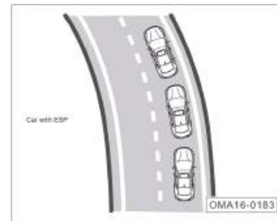
Vehicle equipped with ESP can correct the brakeforce according to the sideslip amount to prevent deviating from the route.
