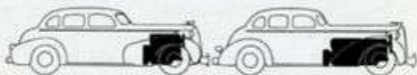
A V-type engine is about six inches shorter than a straight 8 of equal size
