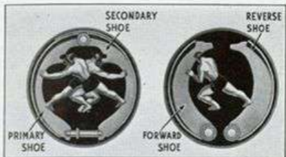
With Duo-Self-Energizing Brakes Both Shoes are Effective
