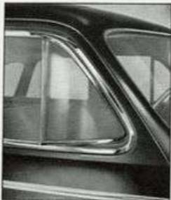
Roof mouldings and ventipane shields protect passengers from dripping water
