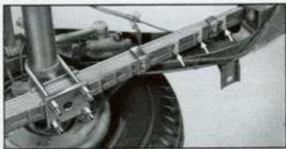
Rear Spring with Waxed Liners
