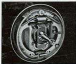
Large Cadillac Hydraulic Brake
