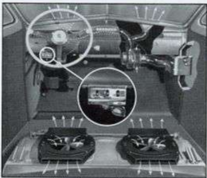
New heating and ventilating system
