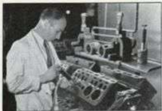
Cylinder bores are graded into one of 30 different sizes with a special expanding gauge.
