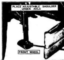
Figure 19. To jack up the car it is necessary to have the jack in the proper position under the axle.
