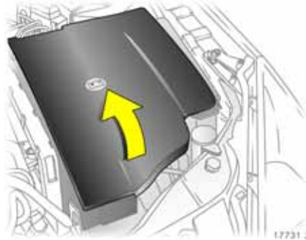
Fuse box in engine compartment The fuse box is in the box at the front left side of the engine compartment.
