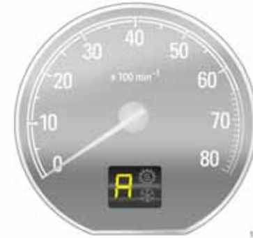
Transmission display Shows the mode or current gear.
