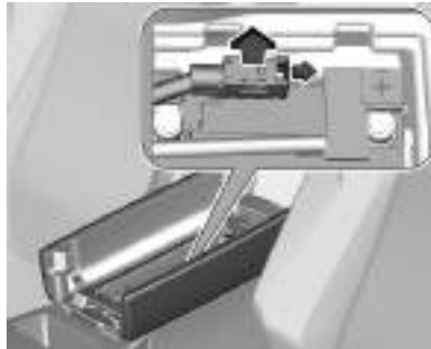
7. Hybrid vehicle: Release and remove connector from negative terminal.
