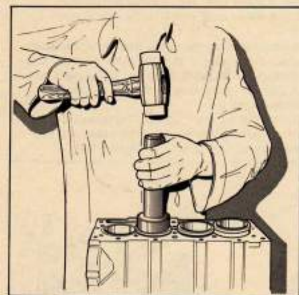
Figure 27 Fitting cylinder liners
