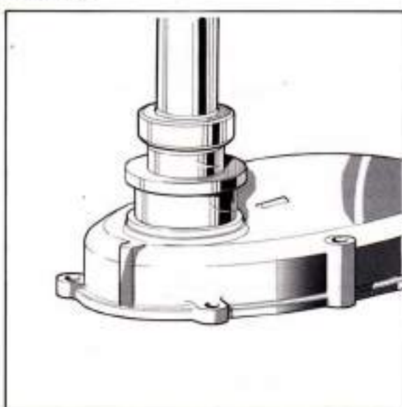
Figure 8 Extracting front cover oil seal
