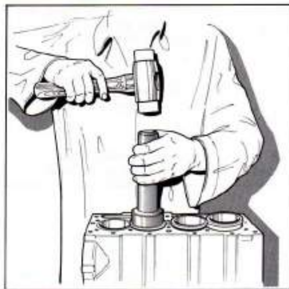
Figure 26 Fitting cylinder liners
