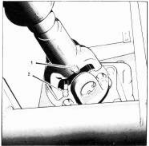
Figure 29 Drive shaft grease nipples
