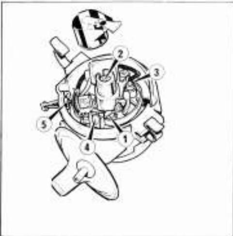
Figure 28 Distributor - general view 1 Locking adjustment screw 4 Terminal post 2 Cam spindle lubrication pad 5 Low tension lead 3 Breaker arm pivot post
