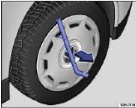
Fig. 190 Pulling the wheel cover off.
