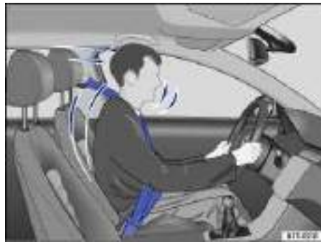
Fig. 62 Belted driver secured by the correctly worn safety belt in the event of a sudden braking maneuver.
