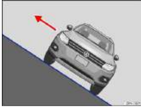
Fig. 161 On a slope, always exit on the uphill side of the vehicle.
