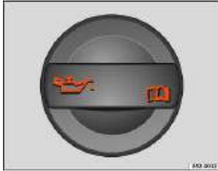
Fig. 165 In the engine compartment: Engine oil filler cap.
