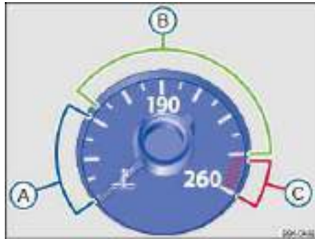
Fig. 166 Engine coolant temperature gauge in the instrument cluster: A Engine cold; B Normal temperature range; C Warning zone.
