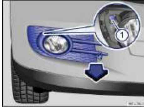
Fig. 202 In right front bumper: Removing light assembly.
