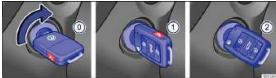
Fig. 134 In the ignition switch: Vehicle key positions.
