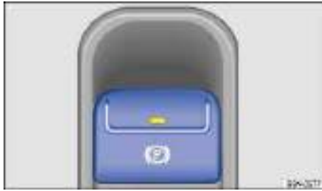
Fig. 142 In the lower center console: Button for the electronic parking brake.
