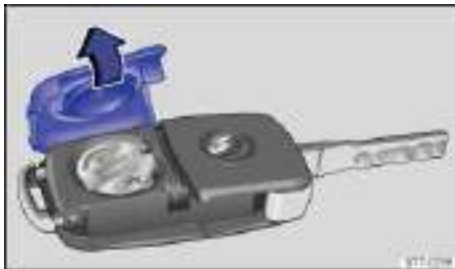
Fig. 23 Remote control vehicle key: Open battery compartment cover.
