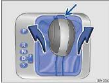
Fig. 182 Removing the selector gate cover.
