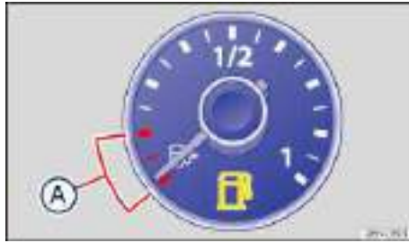
Fig. 156 Fuel gauge in the instrument cluster: A Refuel warning zone.
