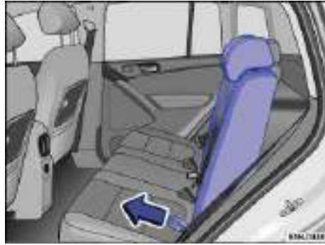
Fig. 97 Folding the backrest forward and back.
