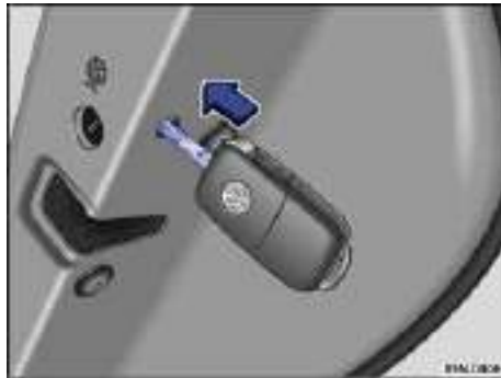
Fig. 180 On the front side of the right rear door: Manual vehicle locking with the key bit in the vehicle key.
