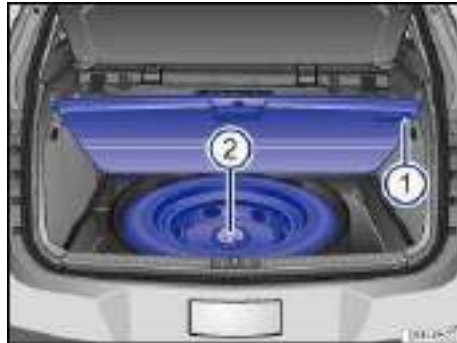
Fig. 114 In the luggage compartment: Compact spare wheel.
