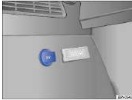
Fig. 132 In the luggage compartment: 12 Volt socket.
