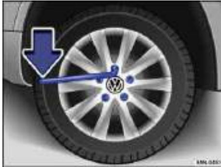
Fig. 191 Changing a wheel: Loosening wheel bolts.
