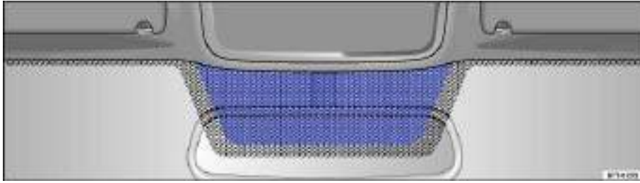
Fig. 87 Heat-reflective windshield with communications window (blue shaded area).
