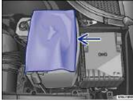
Fig. 170 In the engine compartment: Open the sleeve covering of the vehicle battery.
