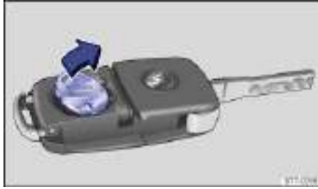
Fig. 24 Remote control vehicle key: Remove old battery.
