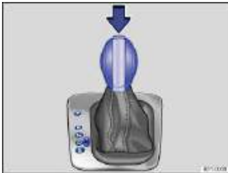
Fig. 140 Automatic transmission selector lever with shift lever release button (arrow).
