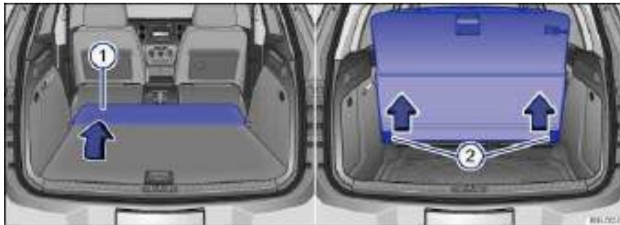
Fig. 106 Extending the luggage compartment floor forward or downward.
