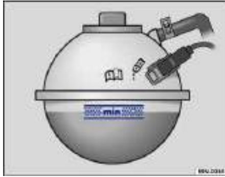
Fig. 167 Coolant expansion tank in the engine compartment.
