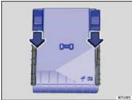
Fig. 197 In the engine compartment: Fuse box cover.
