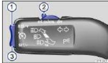
Fig. 149 On the left side of the steering column: Cruise control buttons and switches.
