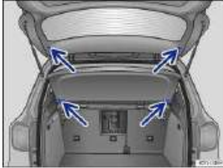
Fig. 100 Installing and removing the luggage compartment cover.
