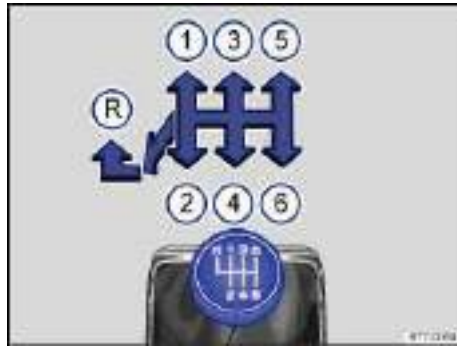
Fig. 139 Gearshift pattern of a 6-speed manual transmission.
