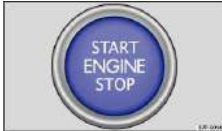
Fig. 135 In the center console: Starter button of the Keyless Access locking and starting system.
