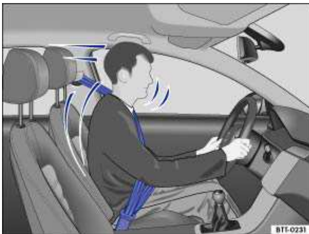
Fig. 54 Belted driver secured by the correctly worn safety belt in the event of a sudden braking maneuver.
