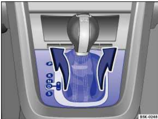
Fig. 177 Removing the selector gate cover.
