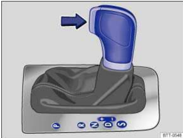
Fig. 133 Side view: Automatic transmission selector lever with shift lever release button (arrow).
