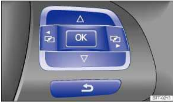
Fig. 16 Right side of the multi-function steering wheel (if applicable): Controls for the menus in the instrument cluster.
