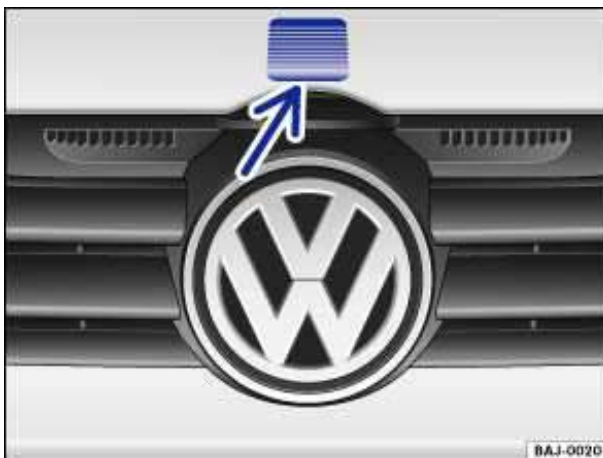
Fig. 154 Above the radiator grille: Outside engine hood release.
