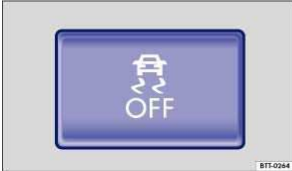
Fig. 137 In the center console: Button for switching ASR on and off manually.
