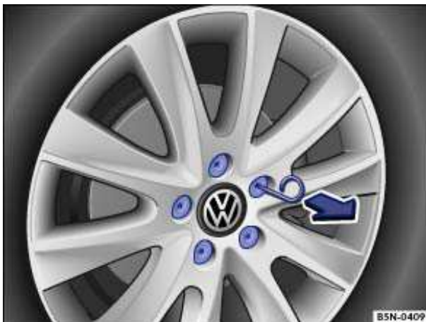
Fig. 185 Pulling cover caps off wheel bolts.
