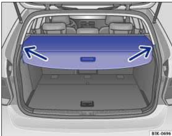
Fig. 98 In the luggage compartment: Closing the luggage compartment cover.
