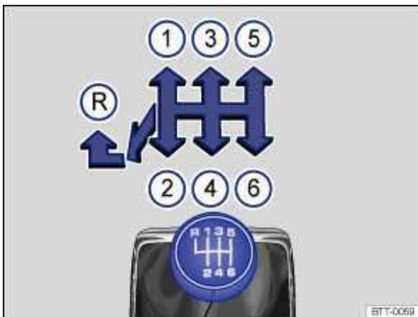
Fig. 132 Gearshift pattern of a 6-speed manual transmission.
