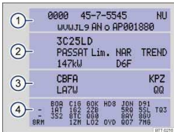
Fig. 17 Vehicle identification label: shown in the example with engine identification code CBFA 3.
