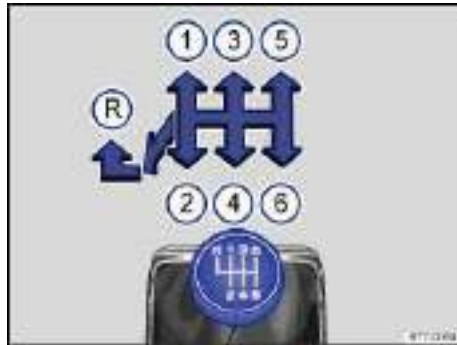
Fig. 134 Gearshift pattern of a 6-speed manual transmission.
