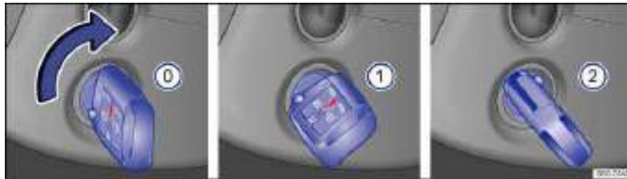
Fig. 127 In the ignition switch: Vehicle key positions.
