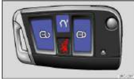
Fig. 22 Remote control vehicle key with panic button.
