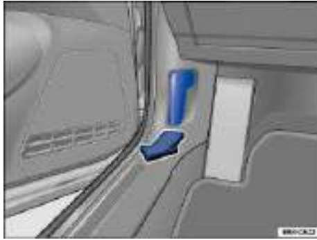
Fig. 165 In the footwell on the driver side: Inside engine hood release lever.
