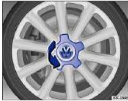
Fig. 188 Twisting the hubcap off.
