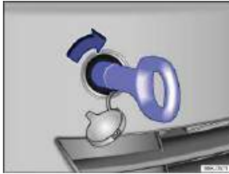
Fig. 203 In the right front bumper: Installing the towing eye.
