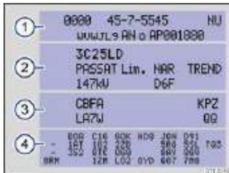
Fig. 16 Vehicle identification label: Shown in the example with engine identification code CBFA 3.
