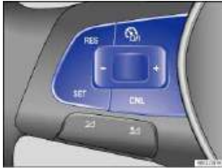
Fig. 144 Left-hand side of the multi-function steering wheel: Buttons for operating the cruise control.
