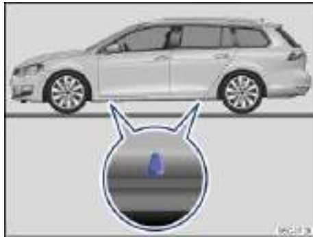
Fig. 192 Lift points for the jack.
