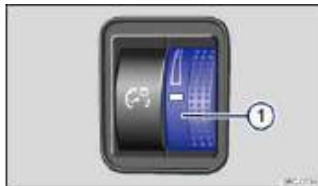
Fig. 77 To the left of the steering wheel: Thumbwheel to adjust instrument panel lighting 1.
