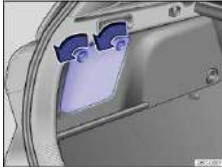
Fig. 184 In the luggage compartment: Opening the side storage compartment.
