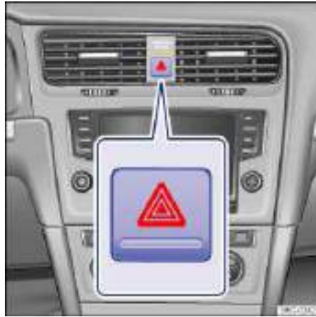
Fig. 176 In the center of the instrument panel: Button for the emergency flashers.
