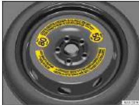
Fig. 109 In the luggage compartment: Compact spare wheel (if equipped).
