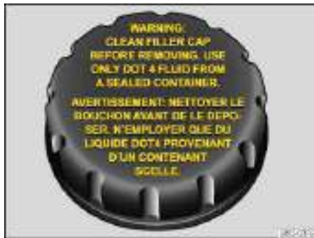
Fig. 140 In the engine compartment: Brake fluid reservoir cap (cap design may vary depending on vehicle equipment).
