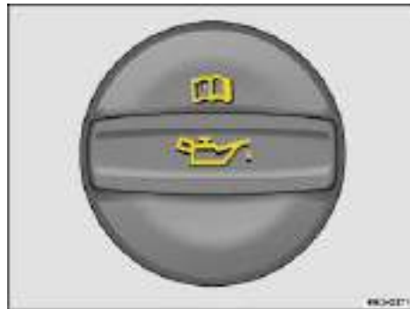
Fig. 168 In the engine compartment: Engine oil filler cap.
