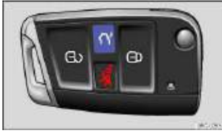
Fig. 28 In the remote control vehicle key: Button to unlock the rear hatch.
