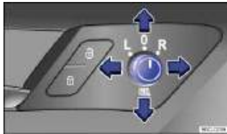
Fig. 88 In the driver door: Adjusting knob for the outside mirrors.
