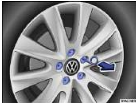
Fig. 189 Pulling cover caps off wheel bolts.
