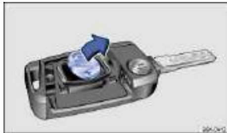
Fig. 21 Remote control vehicle key: Remove old battery.
