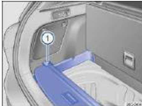
Fig. 93 Under the variable luggage compartment floor: Stowing the luggage compartment cover.
