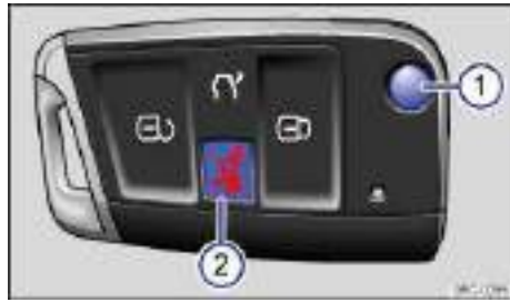
Fig. 18 Remote control vehicle key with panic button.
