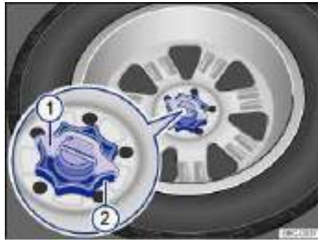
Fig. 108 In the luggage compartment: Handwheel holding the spare wheel in place.
