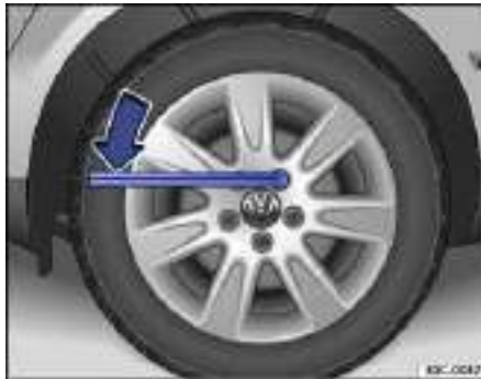
Fig. 191 Changing a wheel: Loosening the wheel bolts.
