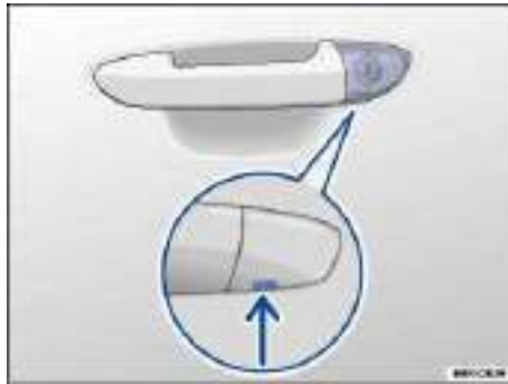
Fig. 177 Door handle on driver door: Concealed lock cylinder (if applicable).
