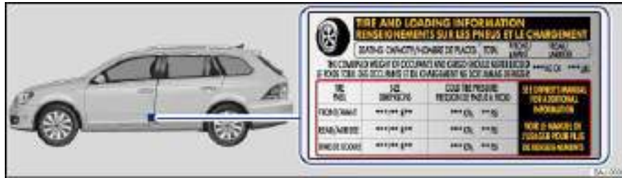
Fig. 106 On the driver door jamb: Location of the tire inflation pressure label.
