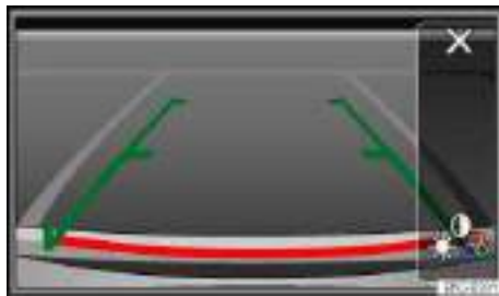
Fig. 147 In the Infotainment system: Rear View Camera system display (display may vary depending on vehicle equipment).
