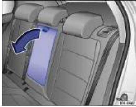
Fig. 46 Folding down the rear center armrest (arrow).
