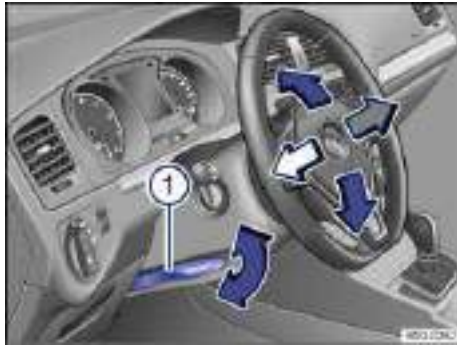
Fig. 44 Manual adjustment for the steering wheel position.
