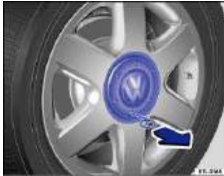
Fig. 187 Pulling the hubcap off.
