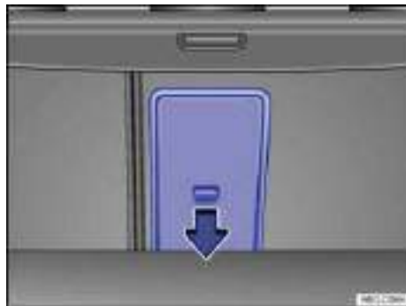
Fig. 95 In the luggage compartment: Opening the pass-through.
