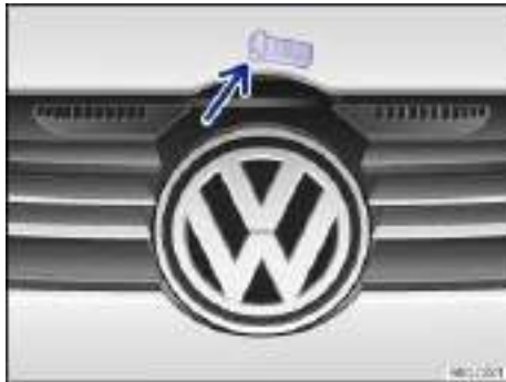
Fig. 166 Above the radiator grille: Outside engine hood release.
