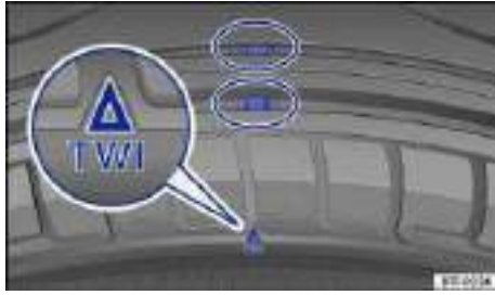
Fig. 107 Tread pattern: Wear indicator.
