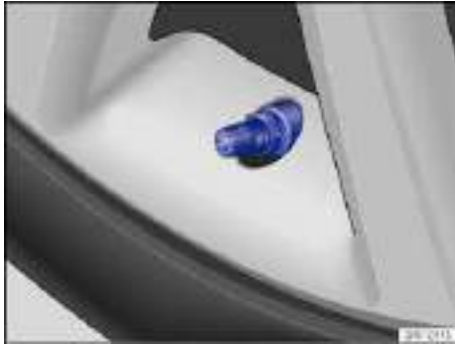
Fig. 108 The Tire Pressure Monitoring system (TPMS) uses a pressure sensor in each read wheel.
