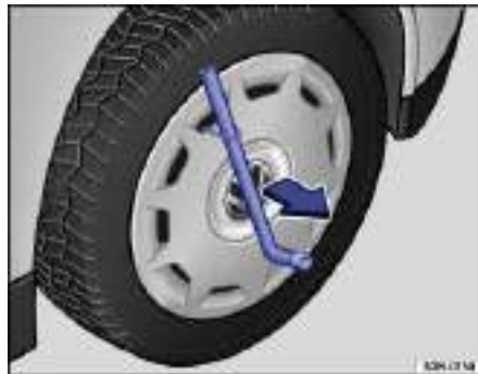
Fig. 183 Pulling the wheel cover off.
