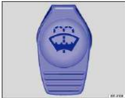
Fig. 91 In the engine compartment: Cap of the windshield washer fluid reservoir.
