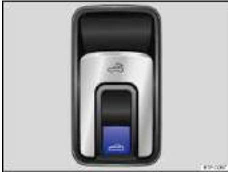
Fig. 37 In the center console: Switch for the power sunroof.
