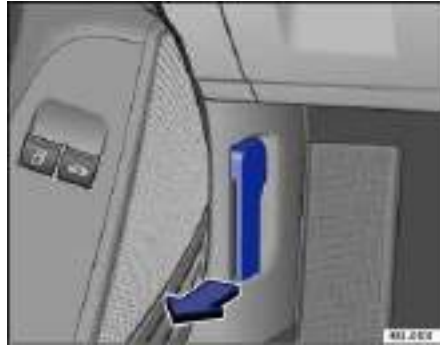
Fig. 150 In the footwell on the driver side: Inside engine hood release lever.
