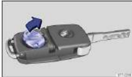
Fig. 22 Remote control vehicle key: Remove old battery.
