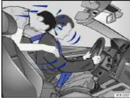
Fig. 57 Unbelted passengers in the rear seats are thrown forward on top of the belted driver.
