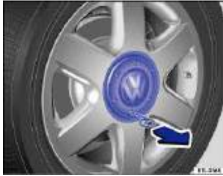
Fig. 180 Pulling the hubcap off.
