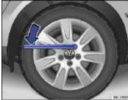
Fig. 184 Changing a wheel: Loosening wheel bolts.
