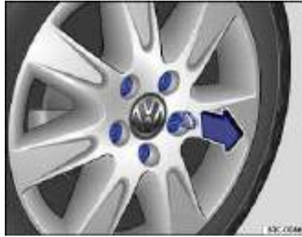
Fig. 182 Pulling cover caps off wheel bolts.
