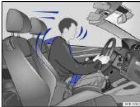
Fig. 58 Belted driver secured by the correctly worn safety belt in the event of a sudden braking maneuver.
