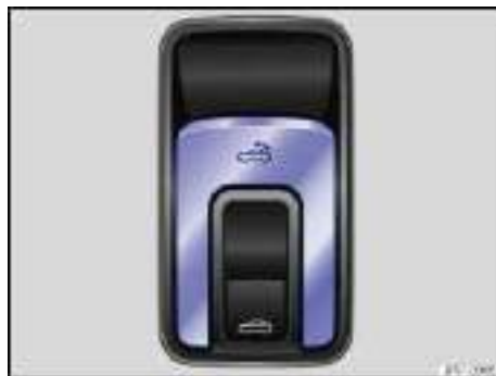
Fig. 172 CSC roof switch in the center console.
