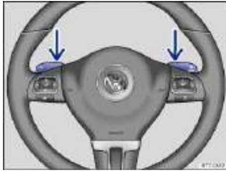
Fig. 131 Steering wheel with optional Tiptronic shift paddles.
