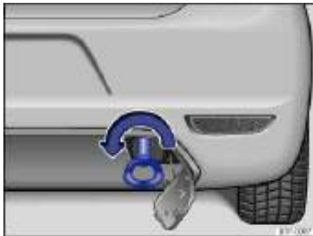
Fig. 201 On the right rear bumper: Screwed-in towing eye.
