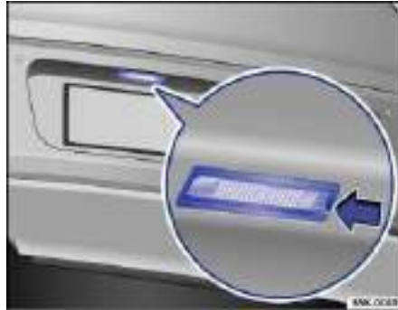
Fig. 195 In the rear bumper: License plate light.
