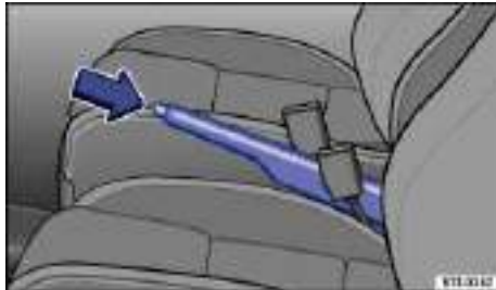
Fig. 132 Between the front seats: Parking brake.
