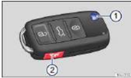
Fig. 18 Remote control vehicle key with panic button.
