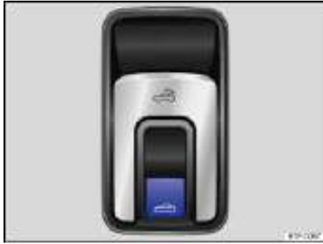
Fig. 35 In the center console: Switch for the power sunroof.
