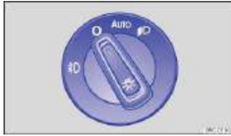
Fig. 83 Headlight switch next to the steering wheel.
