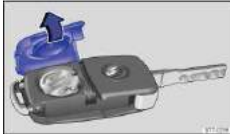
Fig. 21 Remote control vehicle key: Open battery compartment cover.
