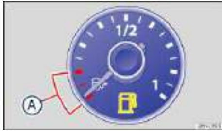
Fig. 147 In the instrument cluster: Fuel gauge.
