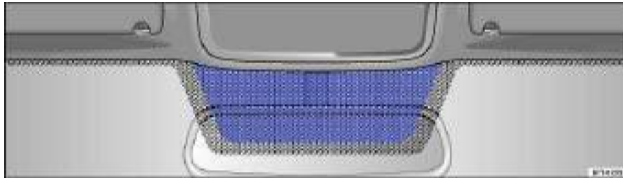
Fig. 86 Heat-reflective windshield with communications window (blue shaded area).
