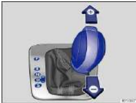
Fig. 130 Selector lever in Tiptronic position.
