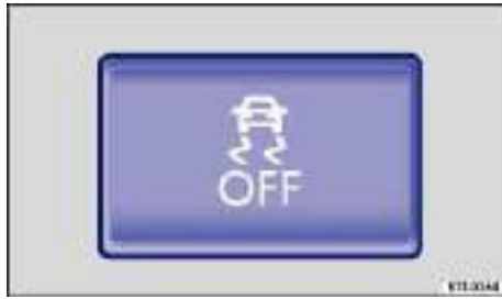
Fig. 133 In the center console: Button for switching ASR on and off manually.
