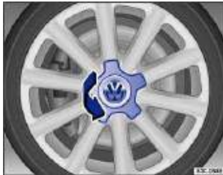
Fig. 181 Twisting the hubcap off.
