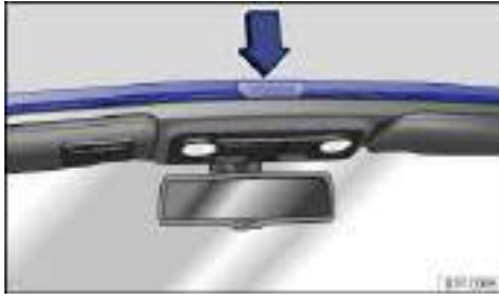
Fig. 36 Wind deflector in the windshield frame.
