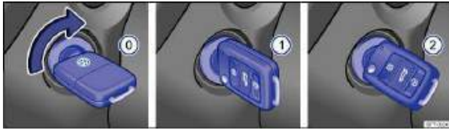
Fig. 124 In the ignition switch: Vehicle key positions.
