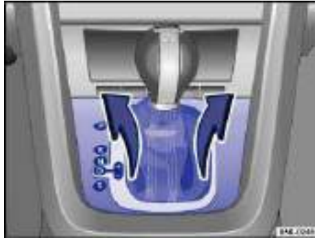
Fig. 175 Removing the selector gate cover.
