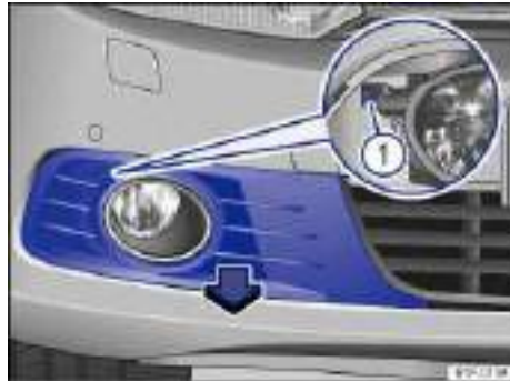
Fig. 193 In front right bumper: Removing the light assembly.
