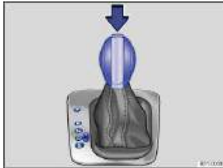
Fig. 129 Automatic transmission selector lever with shift lever release button (arrow).
