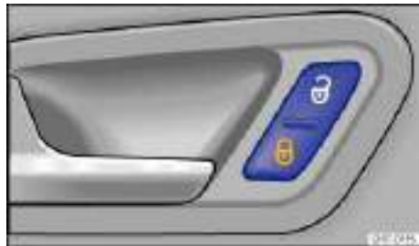
Fig. 24 In the vehicle doors: Power locking button.
