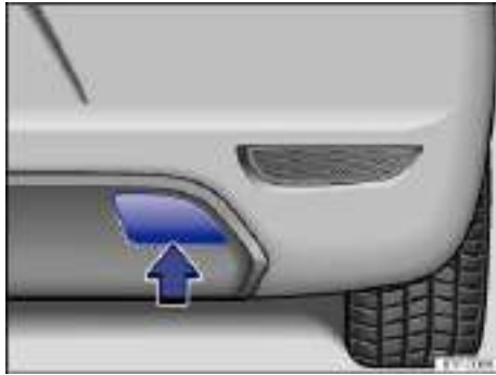
Fig. 200 In right rear bumper: Remove cover.
