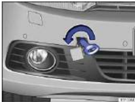
Fig. 199 In right front bumper: Screwing in towing eye.
