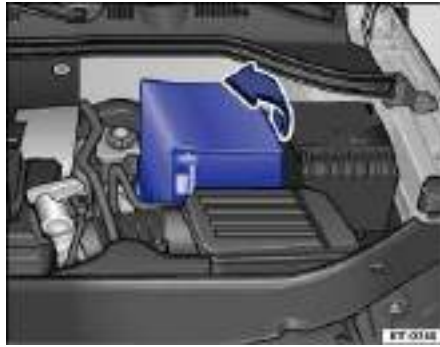
Fig. 158 In the engine compartment: Open the sleeve covering of the vehicle battery.
