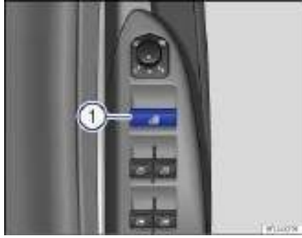
Fig. 173 Driver's door control to open and close all windows.
