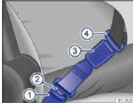
Fig. 63 A safety belt extender properly attached to the factory-installed safety belt.
