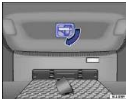
Fig. 168 Inside the luggage compartment: Release lever for luggage compartment lid.
