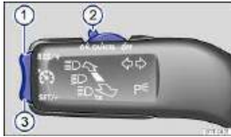
Fig. 139 On the left side of the steering column: Cruise control buttons and switches.
