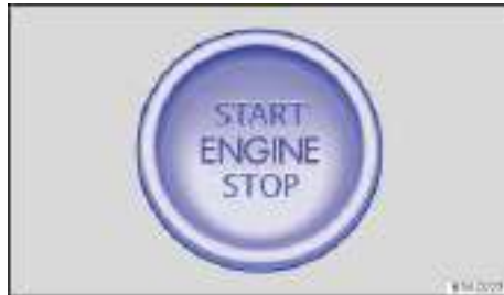
Fig. 125 On the right side of the steering column: Starter button for the Keyless Access locking and starting system.
