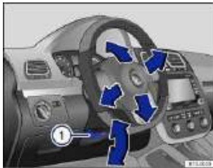
Fig. 48 Manual adjustment for the steering wheel position.
