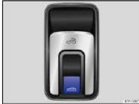
Fig. 171 In the center console: Switch for the power sunroof.
