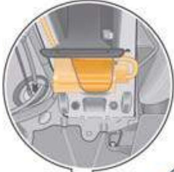
Airbag control unit J234, beneath the centre console
