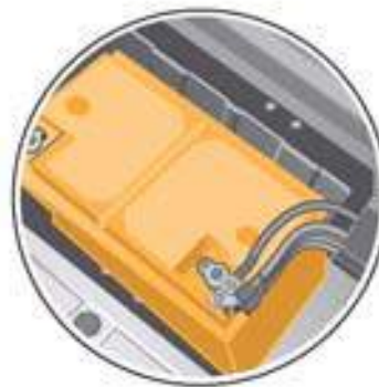
Fuse holder (SA), on right-hand side of battery, visible only following removal
