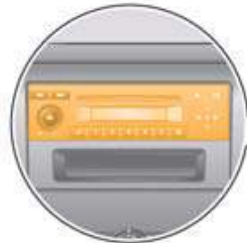
Radio R/control unit with display for radio and navigation J503 *, in centre of dash panel
