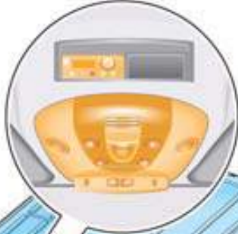
Auxiliary heater control unit J364, in moulded headlining near to the interior mirror
