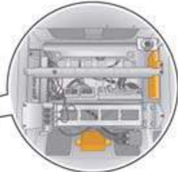
Tyre pressure monitor control unit J502, beneath the front left seat
