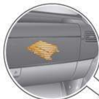
Mobile telephone operating electronics control unit J412, behind the glove box
