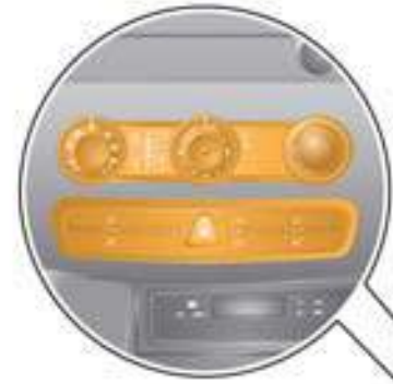
Control unit for middle of dash panel J819, in centre of dash panel
