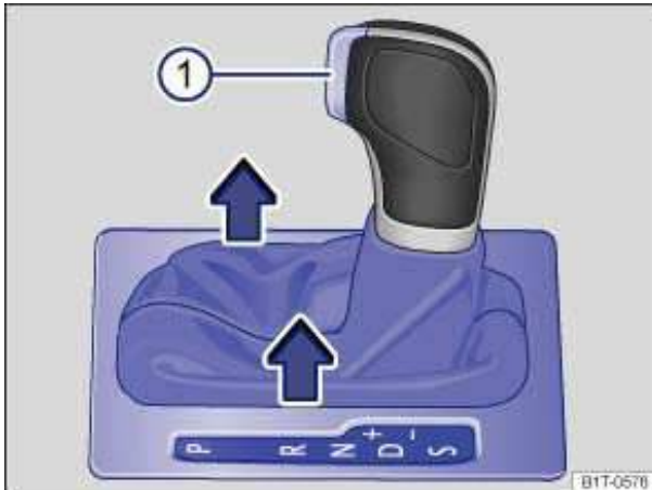
Fig. 167 Removing the selector gate cover.
