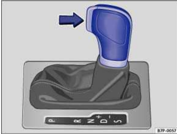
Fig. 117 Side view: Automatic transmission selector lever with shift lever release button (arrow).
