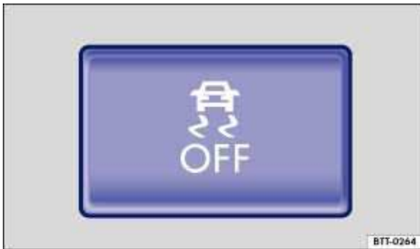
Fig. 122 In the center console: Button for switching ASR on and off manually.
