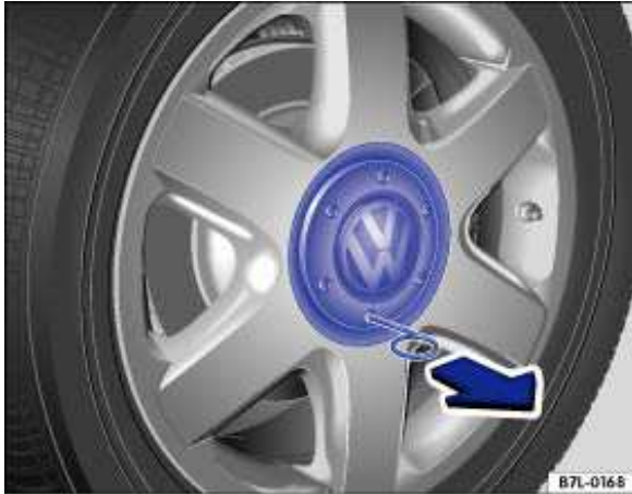
Fig. 171 Pulling the hubcap off.
