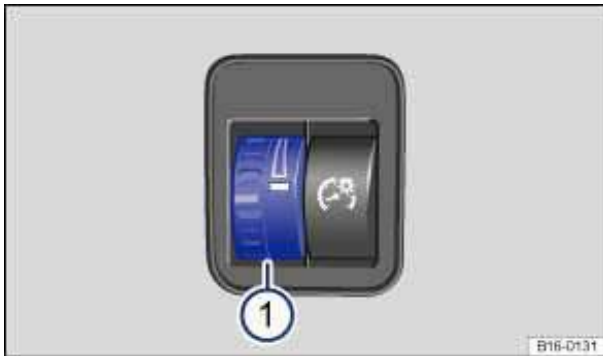
Fig. 74 To the left of the steering wheel: Thumbwheel to adjust instrument panel lighting 1.
