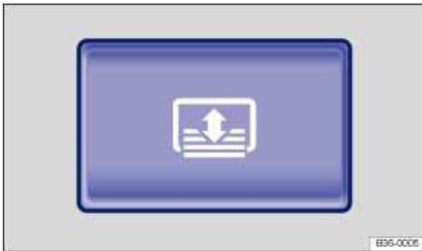
Fig. 77 In the center console: Button for the electrical sunshade on the rear window.
