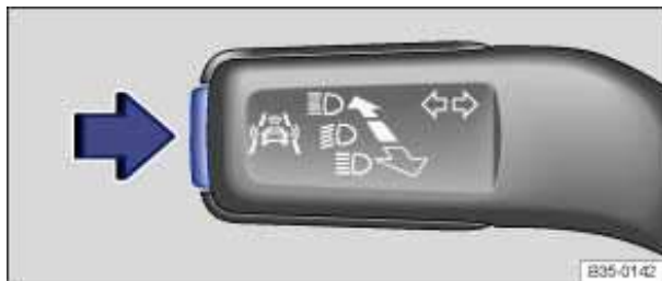
Fig. 13 In the turn signal and high beam lever: Driver assistance systems button.
