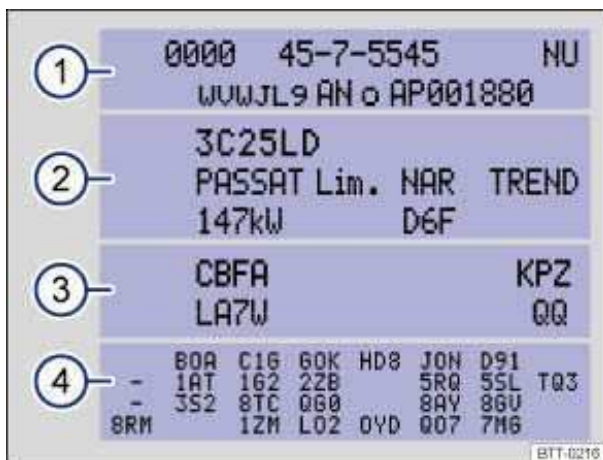
Fig. 14 Vehicle identification label: shown in the example with engine identification code CBFA 3.
