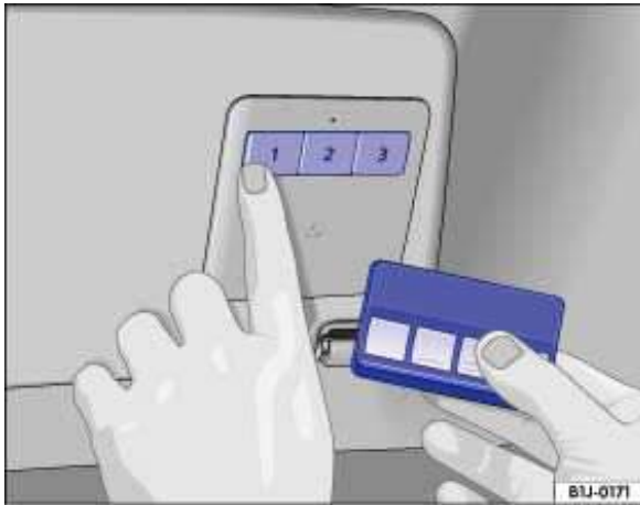
Fig. 30 To program: Simultaneously press the buttons for the HomeLink Universal Transmitter and the remote control.
