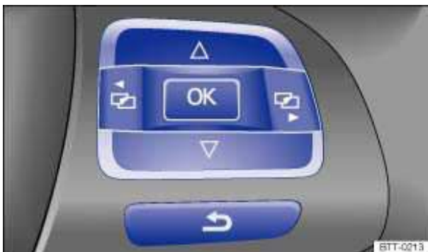
Fig. 12 Right side of the multi-function steering wheel: Controls for menus in the instrument cluster.
