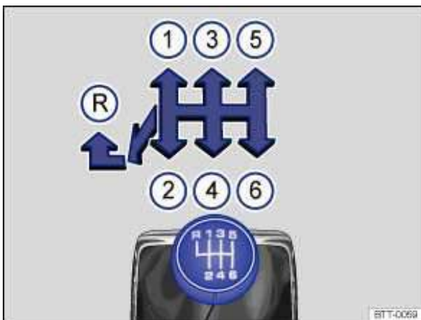
Fig. 99 Gearshift pattern of a 6-speed manual transmission.
