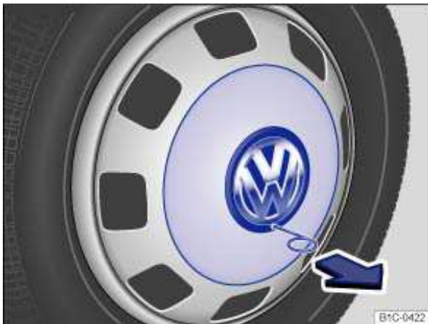
Fig. 140 Pulling the wheel cover off (Version 2).
