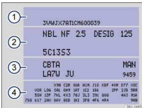
Fig. 15 Vehicle identification label: shown in the example with engine identification code CBTA 3.
