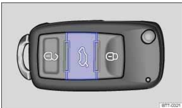
Fig. 25 In the remote control vehicle key: Button to unlock and open the rear hatch.
