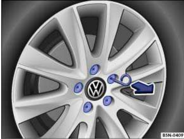
Fig. 141 Pulling cover caps off wheel bolts.
