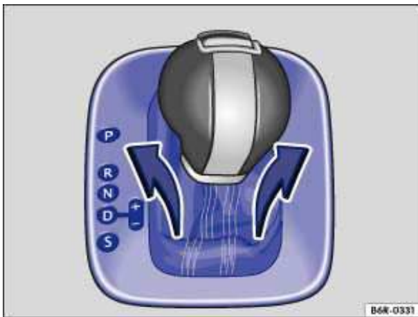
Fig. 133 Removing the selector gate cover.
