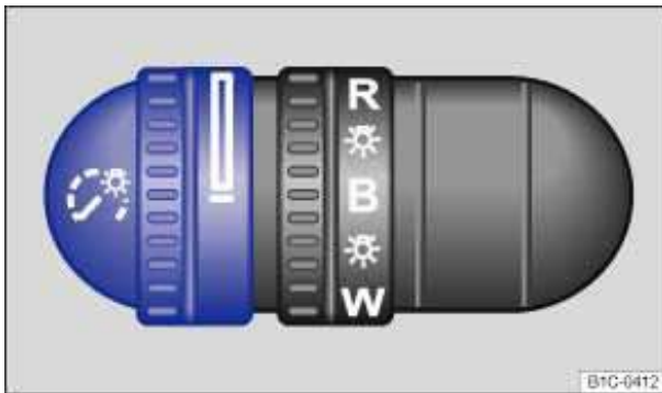
Fig. 67 To the left of the steering wheel: Thumbwheel to adjust instrument panel lighting.
