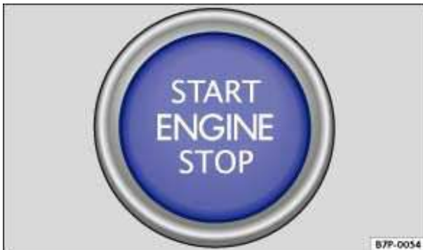
Fig. 94 In the center console: Starter button of the Keyless Access locking and starting system.
