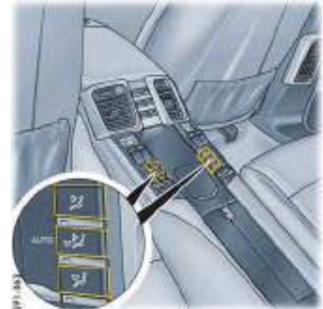
Air distribution, rear control panel (4-zone air conditioning)
