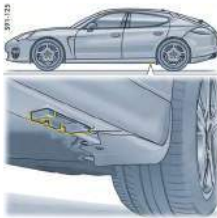
Jacking point for lifting platform and jack at the rear
