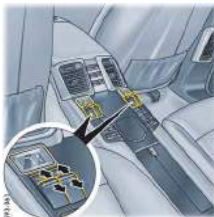
Temperature and air quantity on the rear control panel (4-zone air-conditioning)
