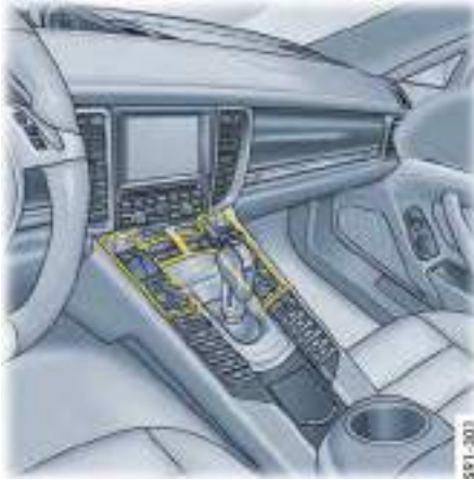
Front air-conditioning control panel
