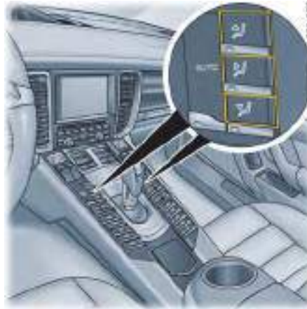
Air distribution, front control panel
