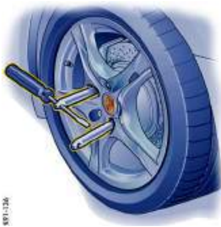
Screw in two assembly aids for cars with Porsche Ceramic Composite Brake
