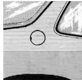
Fuel cap Located in the right rear panel. To close, turn cap clockwise to stop.
