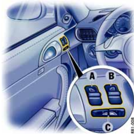
A - Power window in driver's door B - Power window in passenger's door C - Cabriolet: Switching button for front/rear power windows
