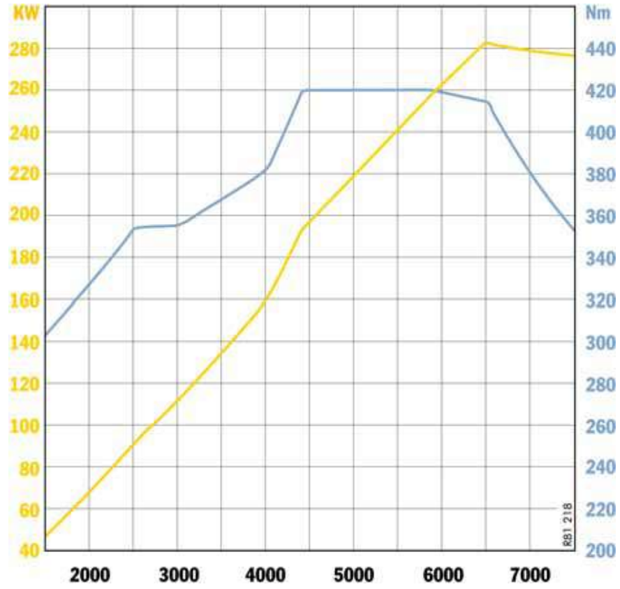
MA 101, Engine diagram at full power, 911 Carrera S, 911 Carrera 4S, 911 Targa 4S
