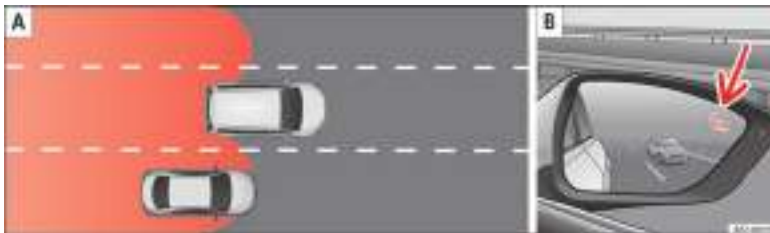
Fig. 205 Schematic diagram: A Situation of passing and then moving into the right-hand lane. B Indication from the blind spot detector in the right-hand external mirror.
