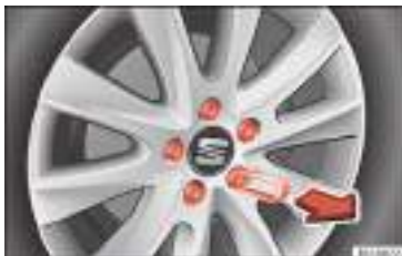
Fig. 70 Wheel: wheel bolts with caps.
