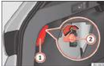
Fig. 110 Luggage compartment: access to the bolt securing the tail light unit.
