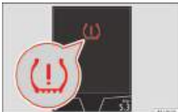
Fig. 240 Instrument panel: warning of loss of tyre pressure.
