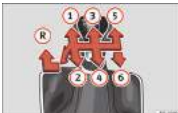
Fig. 52 Gear shift pattern of a 5 or 6-speed manual gearbox.
