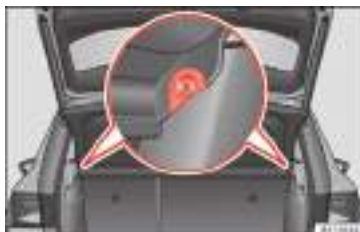
Fig. 155 In the luggage compartment: removing and installing the rear shelf.
