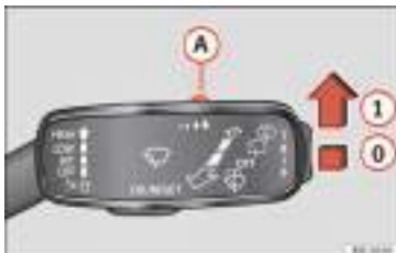
Fig. 143 Windscreen wiper lever: adjusting the rain sensor (A)
