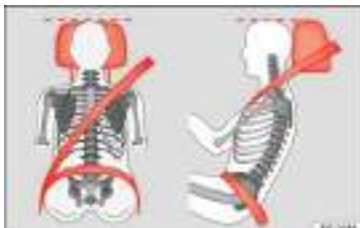
Fig. 17 Correct seat belt and head restraint positions, viewed from front and the side.
