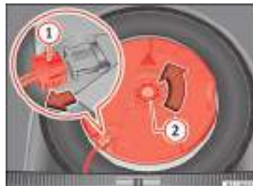
Fig. 242 In the luggage compartment: remove the subwoofer.
