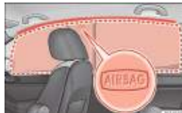
Fig. 27 Location of head-protection airbags.
