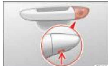
Fig. 3 Driver door lever: hidden lock cylinder.
