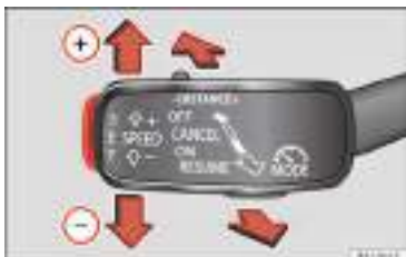
Fig. 48 On the left of the steering column: third lever to operate the CCS.
