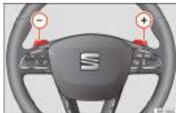
Fig. 175 Steering wheel: automatic gearbox levers
