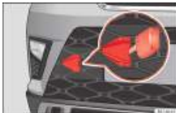
Fig. 97 Front bumper on right: remove the lid.
