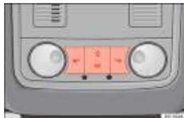
Fig. 38 Detail of headliner: front interior lighting.
