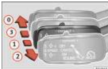
Fig. 186 On the left of the steering column: third lever for operating the Adaptive Cruise Control.
