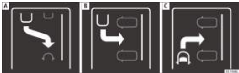
Fig. 213 Overview of reduced displays for parking modes: [A] Parallel parking in reverse. [B] Perpendicular parking in reverse. [C] Perpendicular parking forwards.
