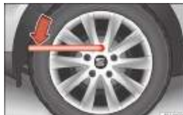
Fig. 72 Wheel: loosen the wheel bolts.
