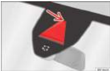
Fig. 199 In the windscreen: field of vision of the Lane Assist system camera.
