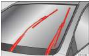
Fig. 79 Wipers in service position.
