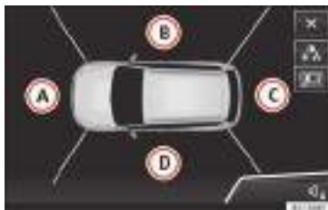
Fig. 225 Display of the Area View system: aerial view.
