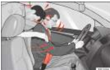
Fig. 90 The unbelted passenger in the rear seat is thrown forward violently, hitting the driver who is wearing a seat belt.
