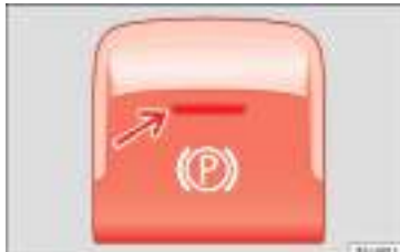
Fig. 172 In the lower part of the centre console: electronic parking brake button.
