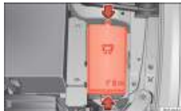
Fig. 65 In the engine compartment: fuse box cover.
