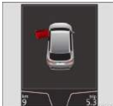
Fig. 50 On the instrument panel display: door open.
