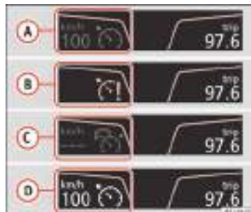
Fig. 178 Instrument panel display: CCS status indications.
