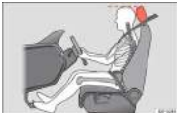
Fig. 83 Correct head restraint position for the driver.
