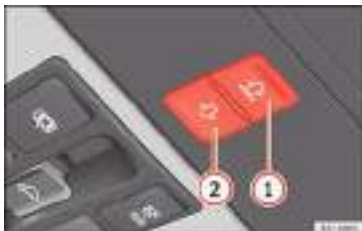
Fig. 137 On the interior roof lining: switches for the sun blind.
