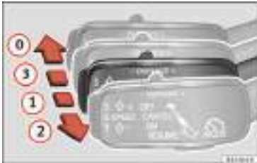
Fig. 188 On the left of the steering column: third lever for operating the Adaptive Cruise Control.
