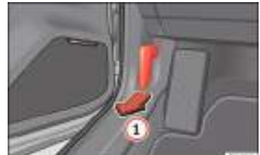
Fig. 9 Release lever in the driver's footwell area.
