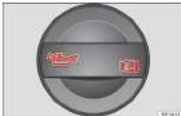
Fig. 236 In the engine compartment: Engine oil filler cap.
