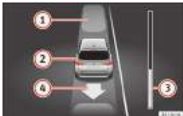
Fig. 217 On the instrument panel display: exiting a parallel parking space.
