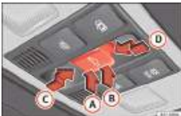
Fig. 136 On the interior roof lining: sunroof button.
