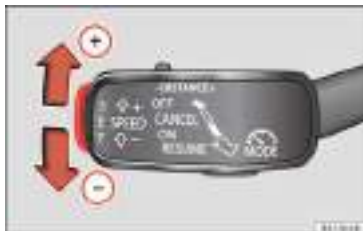
Fig. 187 On the left of the steering column: third lever for operating the Adaptive Cruise Control.
