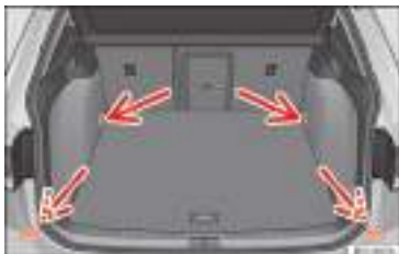
Fig. 160 In the luggage compartment: fastening rings
