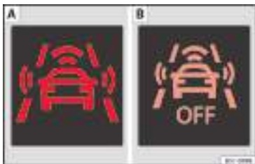
Fig. 196 On the instrument panel display: A Advance warning message. B Pedestrian Monitoring deactivated.
