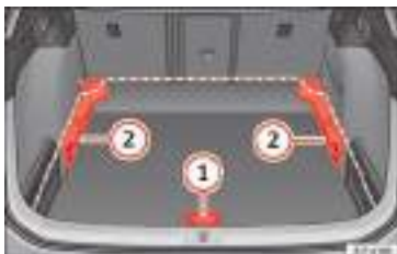
Fig. 164 Luggage compartment variable floor: positions.
