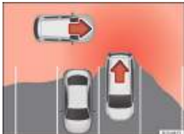
Fig. 206 Schematic representation of the rear cross traffic alert: zone monitored around the vehicle exiting the parking space.
