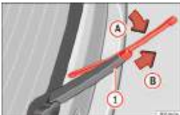
Fig. 81 Changing the rear wiper blade
