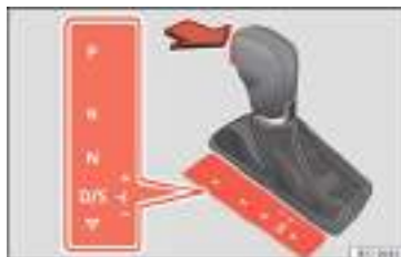
Fig. 53 Automatic gearbox: selector lever positions.
