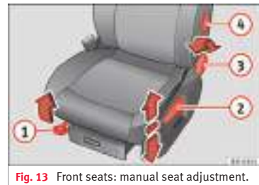
Fig. 13 Front seats: manual seat adjustment.
