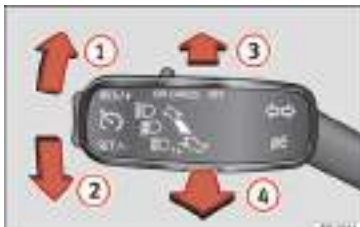
Fig. 36 Turn signal and main beam lever.
