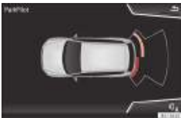
Fig. 223 Parking Aid display on the Easy Connect system screen.
