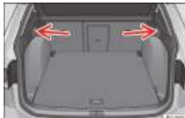
Fig. 161 In the luggage compartment: retaining hooks
