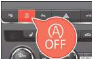
Fig. 176 Centre console: Start-Stop system button.
