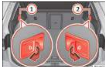
Fig. 149 In the luggage compartment: levers for remote release of the left part (1) and right part (2) of the rear seat backrest.
