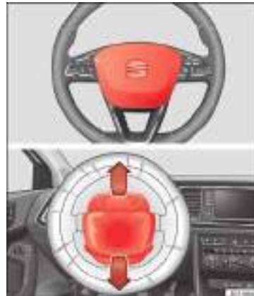
Fig. 20 Driver airbag located in steering wheel.
