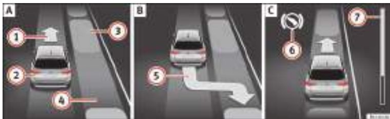
Fig. 215 On the instrument panel display: parallel parking. A Finding a parking space. B Parking position. C Manoeuvring.
