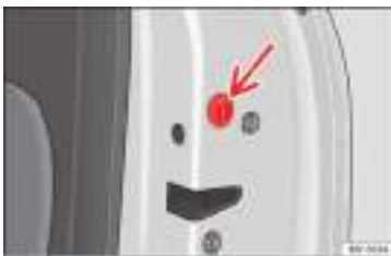
Fig. 4 Locking the door manually.
