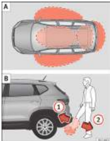
Fig. 127 Keyless Access locking and ignition system: A In the proximity of the car. B Opening the rear lid with sensor-controlled opening (Easy Open)
