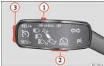
Fig. 180 On the left of the steering column: control and buttons to operate the speed limiter.
