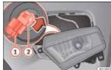
Fig. 109 Fog light: remove the bulb holder.
