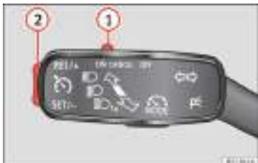
Fig. 47 On the left of the steering column: switches and controls for operating the CCS
