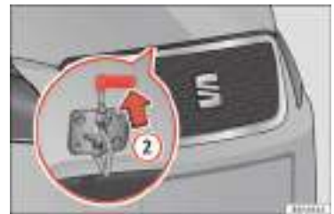
Fig. 10 Cam under the bonnet
