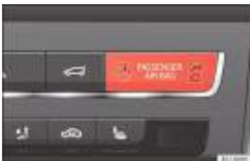
Fig. 51 Warning lamp for disabling the front passenger airbag.
