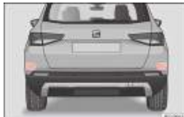
Fig. 203 Rear view of the vehicle: radar sensor zones.
