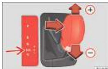
Fig. 174 Centre console: changing gear with tiptronic
