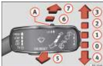
Fig. 39 Operating the windscreen wiper and rear wiper.
