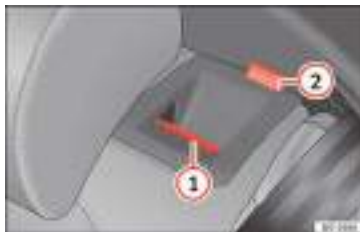
Fig. 148 On the rear seat backrest: release catch (1); red mark (2).
