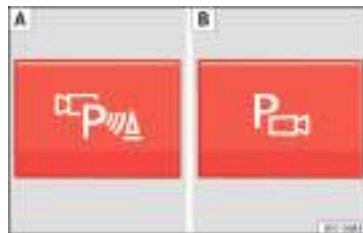
Fig. 226 Centre console: button for activating/deactivating the Area View system manually in combination with the parking aid system (A) or else with the rear ParkPilot system (B).
