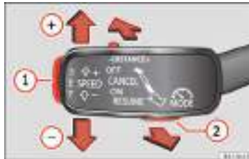
Fig. 181 On the left of the steering column: third lever for operating the speed limiter.
