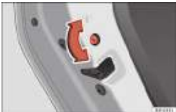
Fig. 131 Childproof lock on the left hand side door.
