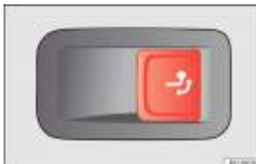
Fig. 230 On the right side of the luggage compartment: button for unlocking the tow hitch.
