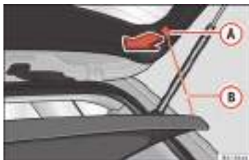
Fig. 154 In the luggage compartment: removing and installing the rear shelf.
