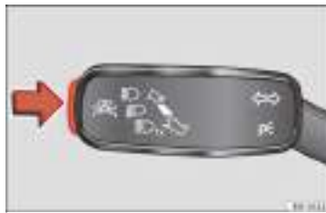
Fig. 44 On the turn signal and main beam headlight lever: button for the driver assistance systems
