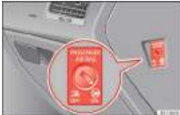
Fig. 22 Front passenger front airbag switch.
