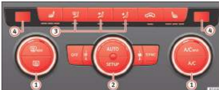
Fig. 55 In the centre console: Climatronic controls
