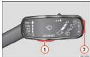
Fig. 42 Windscreen wiper lever: control buttons.
