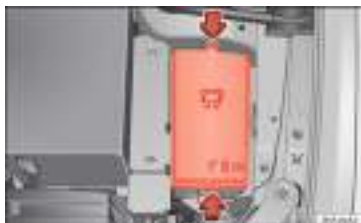
Fig. 103 In the engine compartment: fuse box cover.
