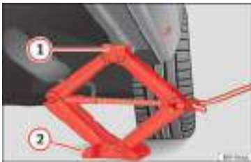
Fig. 74 Strut: mounting the jack on the vehicle.
