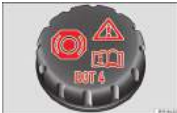
Fig. 62 Engine compartment: brake fluid reservoir cap.
