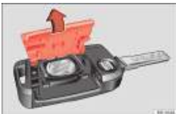
Fig. 129 Vehicle key: opening the battery compartment.
