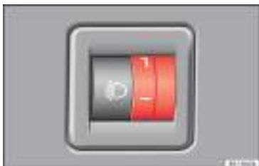
Fig. 141 Next to the steering wheel: Headlight range control
