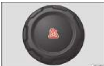
Fig. 61 Engine compartment: coolant expansion tank cap.
