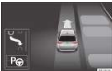
Fig. 214 On the instrument panel display: displaying the Park Assist system with reduced display.
