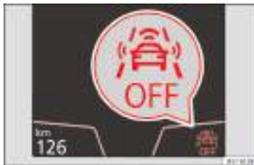
Fig. 194 On the instrument panel display: Front Assist switched off message.
