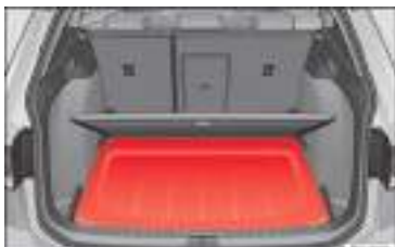
Fig. 157 In the luggage compartment: fitting the storage compartment shelf.
