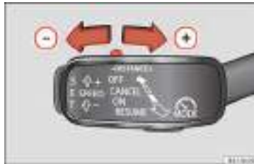
Fig. 189 Control lever: setting the distance.
