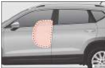
Fig. 26 Illustration of completely inflated side airbags on the left side of the vehicle.
