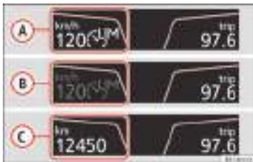
Fig. 179 On the instrument panel display: messages on the status of the speed limiter.
