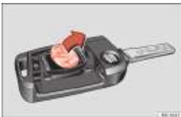
Fig. 130 Vehicle key: removing the battery.
