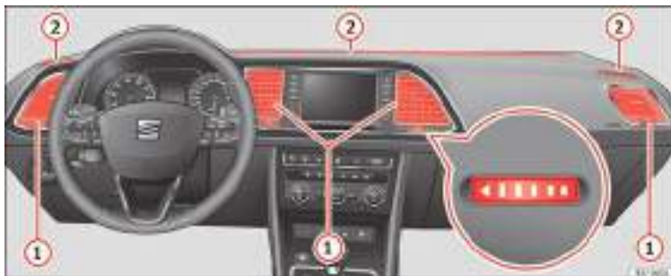
Fig. 167 On the dash panel: air vents
