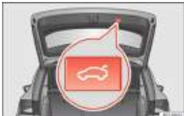
Fig. 133 Rear lid open: button to close the rear lid immediately.
