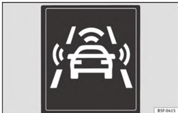
Fig. 195 On the instrument panel display: advance warning message.
