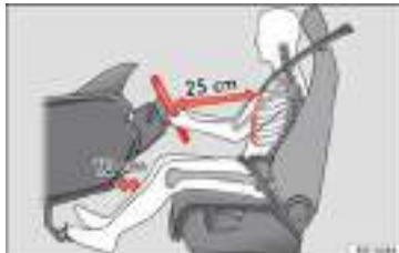
Fig. 82 The proper distance between driver and steering wheel.
