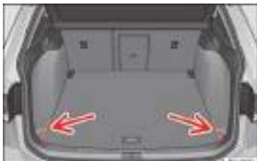
Fig. 156 In the luggage compartment: covers for storing the rear shelf.
