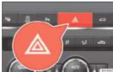
Fig. 37 Dash panel: switch for hazard warning lights.
