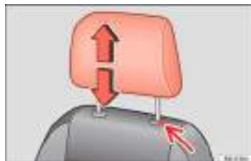
Fig. 76 Adjusting and removing the head restraints.
