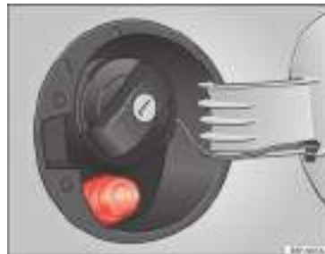
Fig. 143 Fuel tank flap open with EURO-type connector.
