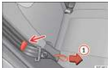
Fig. 81 Folding the rear seat backrests down.
