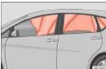
Fig. 18 Deployed head-protection airbags.
