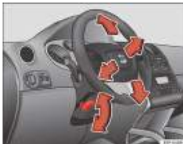
Fig. 3 Adjusting the steering wheel position.
