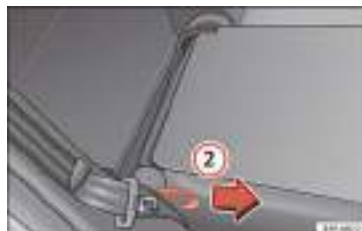
Fig. 82 Lifting the rear seat backrests.
