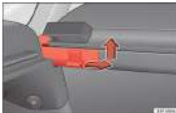
Fig. 106 Removing the storage compartment shelf.
