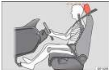
Fig. 2 Correct head restraint position for the driver.
