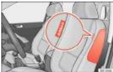
Fig. 15 Side airbag in driver seat.
