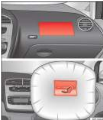
Fig. 14 Front passenger airbag in the dash panel.
