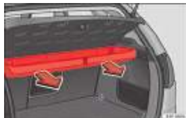
Fig. 104 Removing the storage compartment. »
