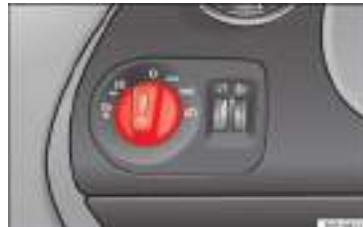
Fig. 58 Detailed view of the dash panel: lights, front fog lights and rear fog light switch.
