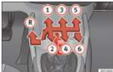
Fig. 124 Detailed view of the centre console: gear shift pattern of a 5- or 6-speed manual gearbox.
