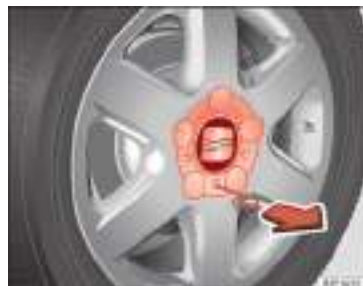
Fig. 155 Changing a wheel: remove the wheel trim.
