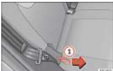
Fig. 80 Rear seat backrest angle adjustment.
