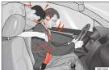
Fig. 9 The unbelted passenger in the rear seat is thrown forward violently, hitting the driver wearing a seat belt.
