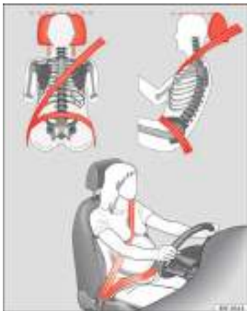
Fig. 11 Placing the seat belt in the shoulder and pelvis area for pregnant women.
