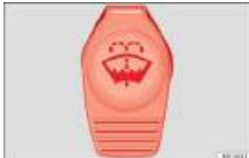
Fig. 150 In the engine compartment: Cap of windscreen washer fluid reservoir
