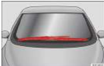
Fig. 169 Windscreen wipers in the service position.
