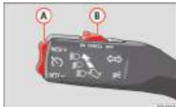
Fig. 135 Turn signal and main beam headlight lever: switch and rocker switch for the cruise control.
