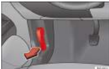
Fig. 144 Detail of footwell area on driver side: lever for unlocking the bonnet
