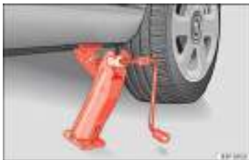
Fig. 159 Fitting the jack.
