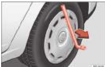
Fig. 156 Changing a wheel: remove the wheel cover.
