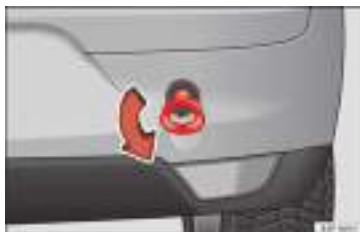
Fig. 166 Fitting the towline anchorage to the rear of the vehicle.
