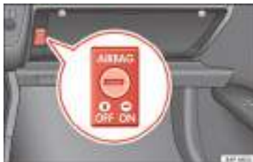
Fig. 19 In the glove compartment: Switch for activating and deactivating the front passenger airbag
