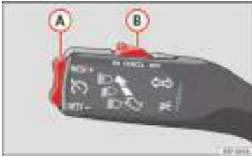
Fig. 136 Turn signal and main beam headlight lever: switch and rocker switch for the cruise control.
