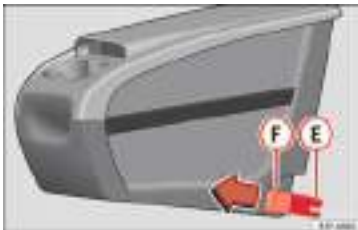
Fig. 93 Mobile storage compartment. Mounting.
