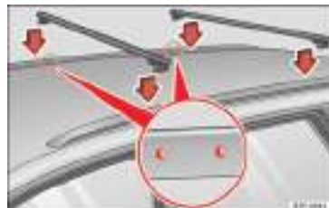
Fig. 113 Altea XL/Altea Freetrack model: securing points for the roof carrier.
