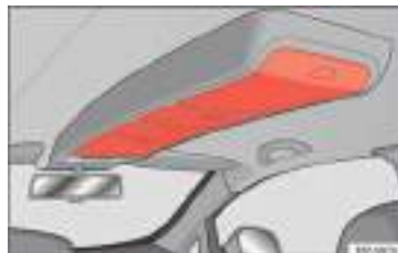
Fig. 87 Roof storage compartments.
