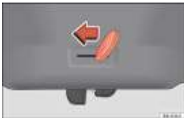
Fig. 168 Rear lid: emergency opening.
