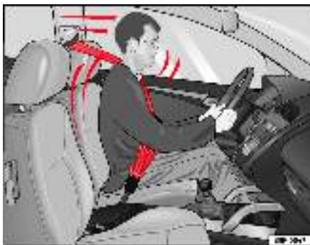
Fig. 9 Driver wearing the seat belt properly: is secured by the belt in sharp braking
