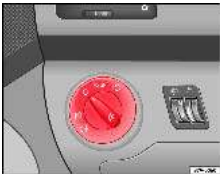
Fig. 70 Detailed view of dash panel lights, fog light and rear fog light control
