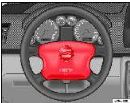
Fig. 22 Driver airbag located in steering wheel
