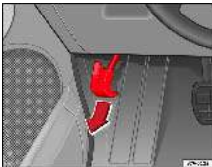
Fig. 137 Detail of footwell area on driver's side: lever for unlocking the bonnet.
