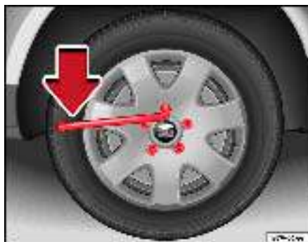
Fig. 157 Changing the wheel: loosen the wheel bolts
