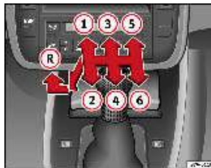
Fig. 126 Manual gearbox with shift diagram
