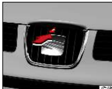
Fig. 138 Detail of radiator grille: lever for unlocking the bonnet.
