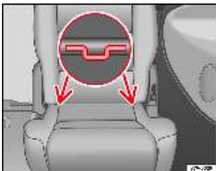
Fig. 33 Retaining rings for ISOFIX child seats in the frames of the outer seats in the second row of seats
