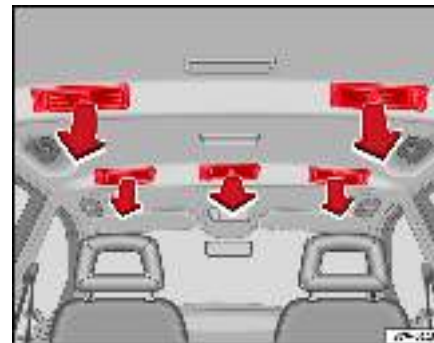
Fig. 121 Cold air vents in the roof
