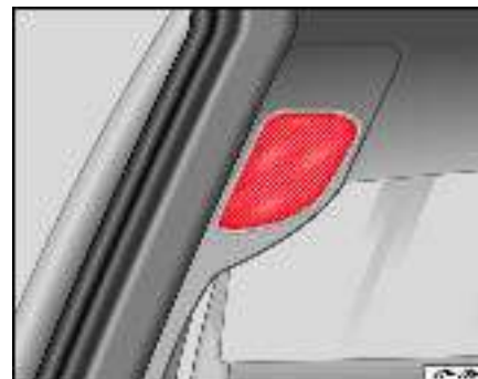
Fig. 62 Interior monitoring system sensor
