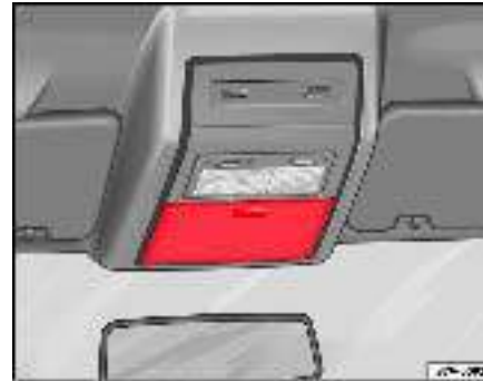
Fig. 103 Stowage area in the roof
