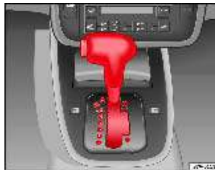
Fig. 127 Centre console: selector lever of the automatic gearbox with locking button
