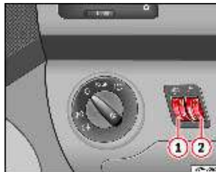
Fig. 71 Instrument panel: headlight range control ① and illumination of instruments and switches ②
