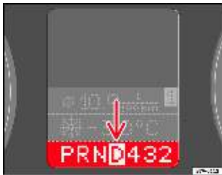
Fig. 128 Instrument panel: display showing position of selector lever
