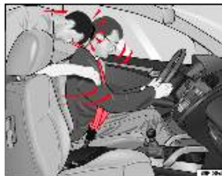
Fig. 8 The unbelted rear passenger is thrown forward violently, hitting the driver wearing a seat belt.
