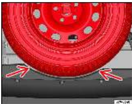
Fig. 152 Resting point for the spare wheel on the bumper
