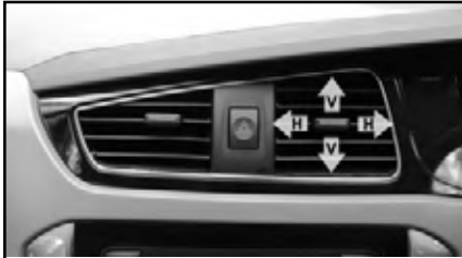
Middle air vent
