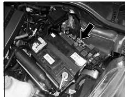
Fuse Box - Engine Compartment
