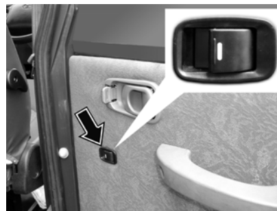
Individual Switches on the rear doors for operating the rear door glasses
