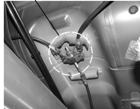
1. Parking Brake Adjustment Nut 2. Check Nut
