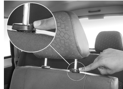
Release Button for Head rest height adjustment
