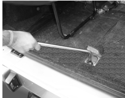
Loosening/Tightening of wheel winch screw
