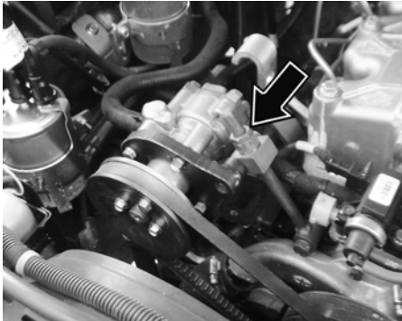
Power Steering Pump Belt Adjustment Nut
