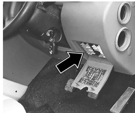
Fuse Box - Cabin
