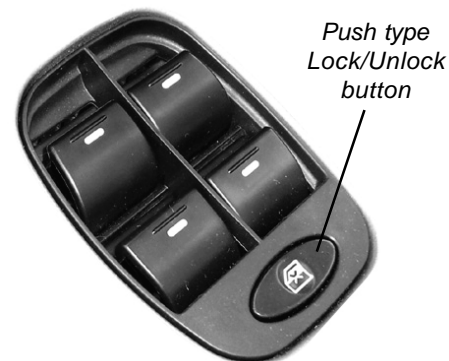
Window Winding Switch
