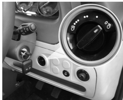
Headlamp Leveling Switch
