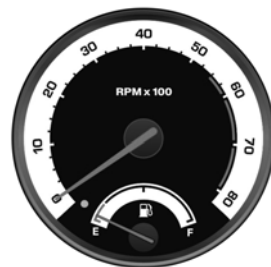
RPM meter (Petrol)
