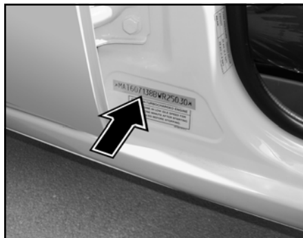
Chassis Number on 'B' pillar
