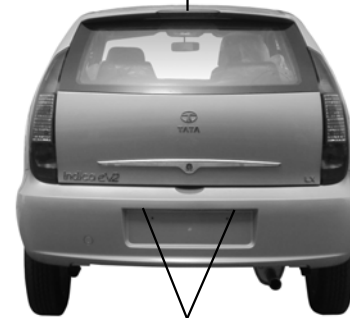
Registration Plate Lamps
