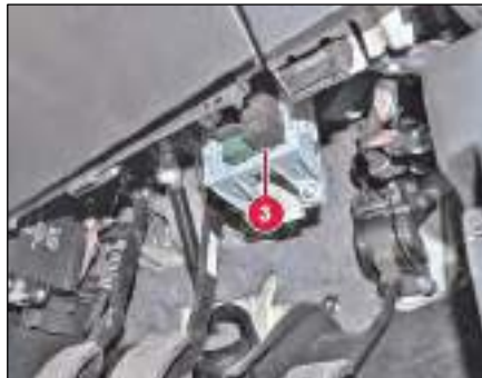
Fuse location- Cabin compartment
