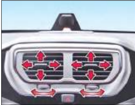
Center air vents
