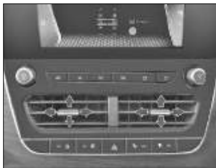
Centre Air Vents (Front)
