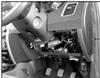
Fuse Box - Cabin Compartment
