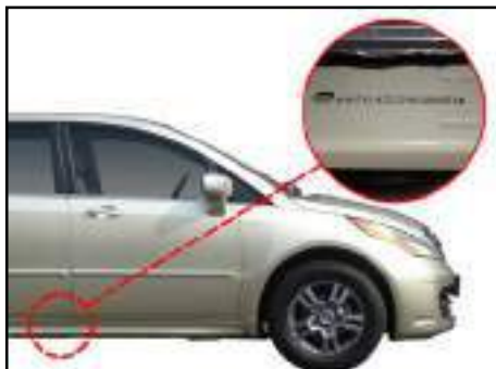
Chassis No. - Punched on RH Long member
