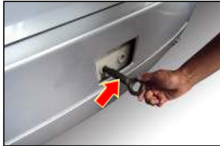
Tow Hook Attachment Location at Rear
