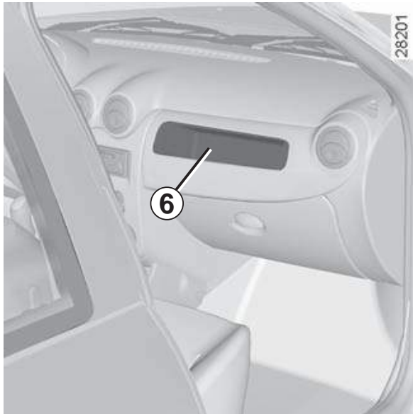
Storage compartment 6 (or passenger air bag location)
