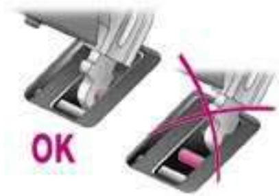
Correct securing of the front feet
