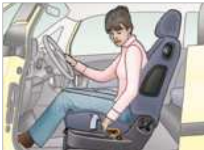
2. Driver's seat height adjustment.
