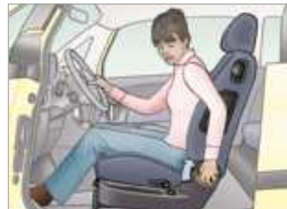
3. Seat back angle adjustment.
