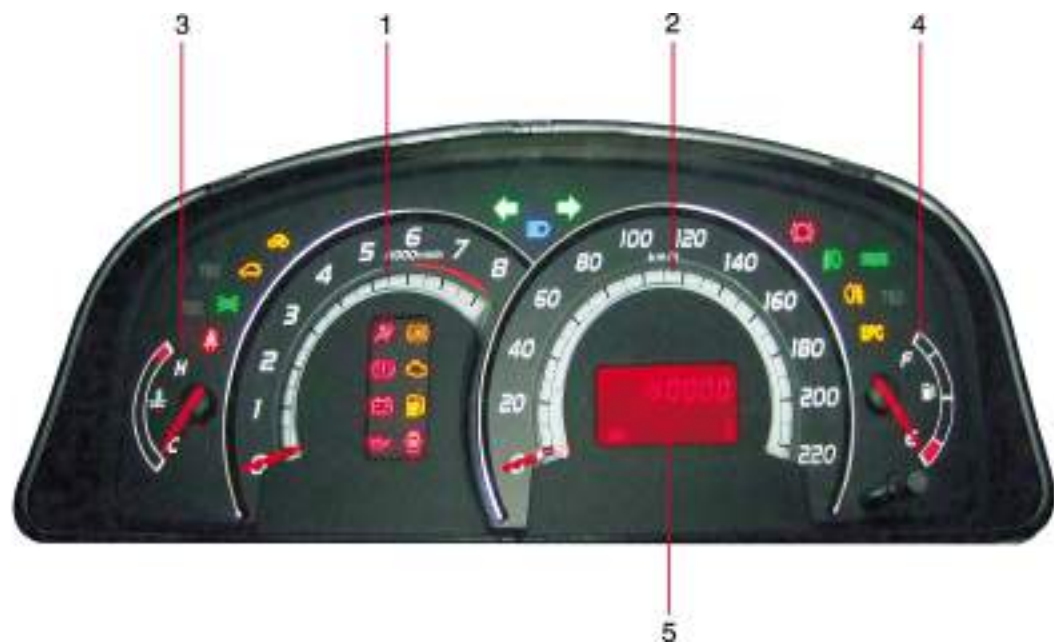
1. Tachometer 2. Car speed meter 3. Thermometer 4. Fuel oil meter 5. Mileage/shift/time indicator light
