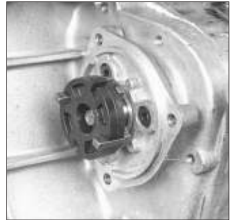
18.6c . . . and on the drive coupling on the auxiliary shaft side; note that the two lugs on each drive coupling fit into their corresponding slots in the coupling disc, 180° apart - all four lugs must be properly engaged or you won't be able to bolt the adapter to the auxiliary shaft housing
