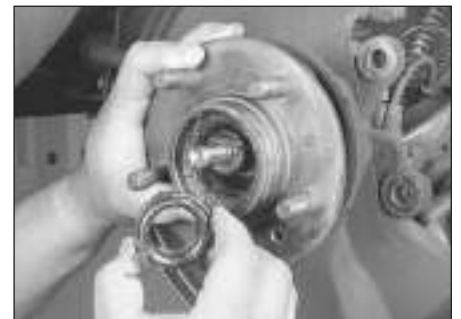
22.9 Pull the hub assembly forward slightly - then push it back into position to dislodge the outer wheel bearing
