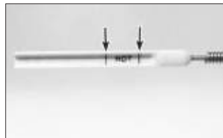
8.4b Check the automatic transmission fluid with the engine idling at operating temperature and the gear selector in Park, then add fluid to bring the level to the upper mark
