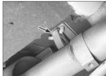
14.1b Check the condition of the flexible rubber mounts that hang the silencer to the chassis
