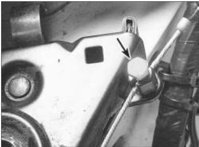
11.1 Remove the cable retaining bolt(s) (arrowed) then disengage the cable from the latch assembly
