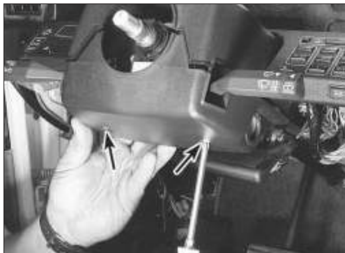
27.3 Remove the lower steering column cover screws
