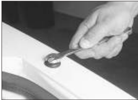
14.1 The aerial mast retaining nut can be removed with an open end spanner
