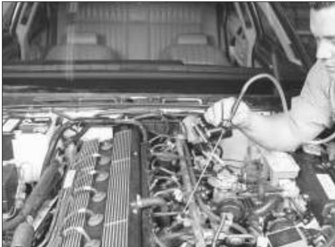
12.7 Use a stethoscope or a screwdriver to determine if the injectors are working properly - they should make a steady clicking sound that rises and falls with engine speed changes
