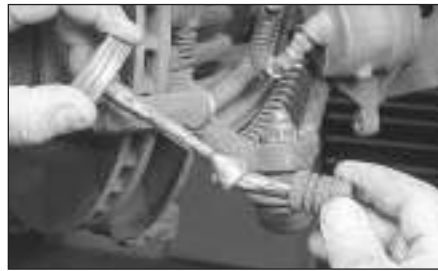
3.5j . . . clean them off, inspect the pin and boot for damage, renew as necessary, then lubricate the pins with brake grease and refit them in the caliper bracket
