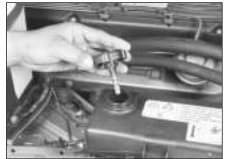
5.7 On 1990 and later models remove the cap and check the fluid level on the dipstick
