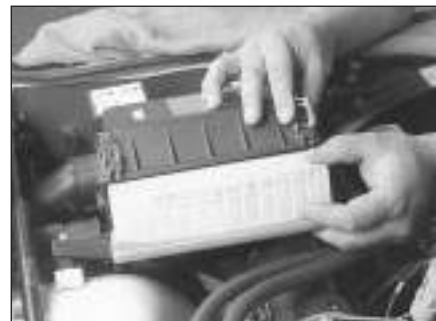
17.1 Detach the clips and separate the cover, then slide the filter element out of the housing
