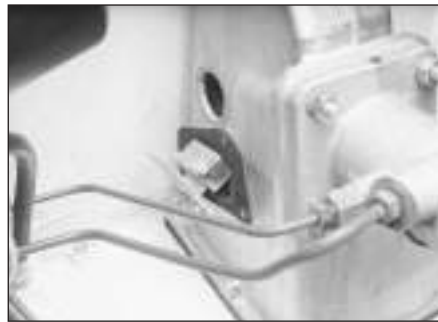
13.6b . . . and carefully pry the switch plate away from the pedal box - be careful not to damage the gasket
