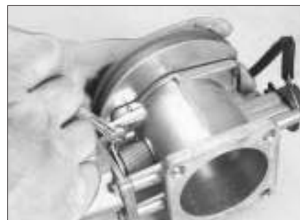
13.20 Adjust the butterfly angle by loosening the locknut on the throttle stop and turning the adjustment bolt
