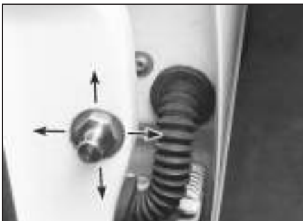
19.13 Adjust the door lock striker by loosening the hex nut and gently tapping the striker in the desired direction
