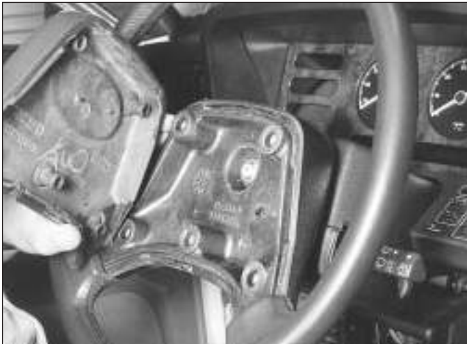
14.2 To remove the centre pad from the steering wheel, simply pry it off
