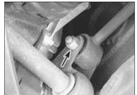
13.7 Remove this nut (arrowed) and bolt from the lower end of each tie-bar (right above the control arm pivot)
