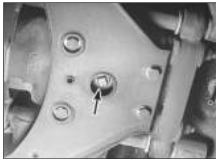
27.4 The differential drain plug (arrowed) is accessible through a hole located in the middle of the differential support brace
