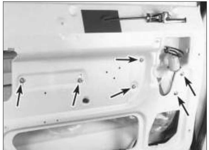
21.3 Detach the window regulator bolts (arrowed)
