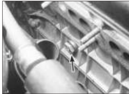
30.5 The block drain plug (arrowed) is located on the right side of the block
