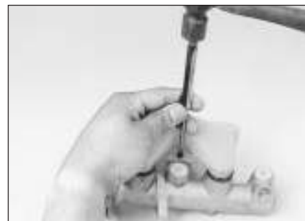
6.7a Knock out the roll pin that secures the reservoir to the master cylinder
