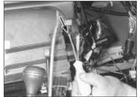
11.6a Remove three screws (one arrowed; one at the top-back and one below) to take out the climate-control computer on right side of heater/air conditioning assembly
