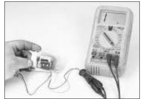
13.7a To check the brake light switch, connect an ohmmeter to the switch terminals; with the switch plunger released, there should be no continuity (infinite resistance)
