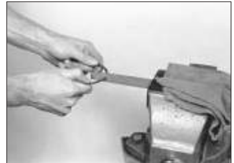
22.5 If the end gap is too small, clamp a file in a vice and file the ring ends (from the outside in only) to enlarge the gap slightly
