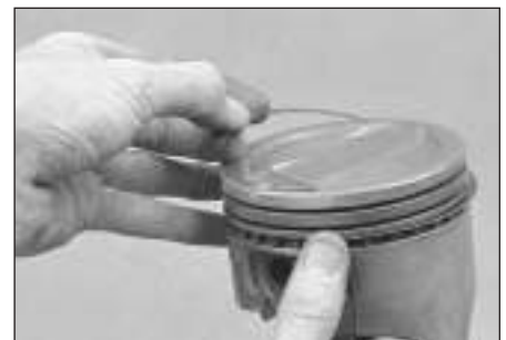
22.9b DO NOT use a piston ring refitting tool when refitting the oil ring side rails
