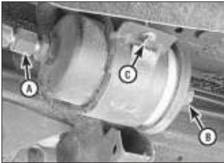
18.3 Remove the banjo bolt from the outlet side (B), detach the fitting from the inlet side (A) and unscrew the filter mounting bolt (C)
