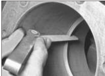
22.4 With the ring square in the cylinder, measure the end gap with a feeler gauge
