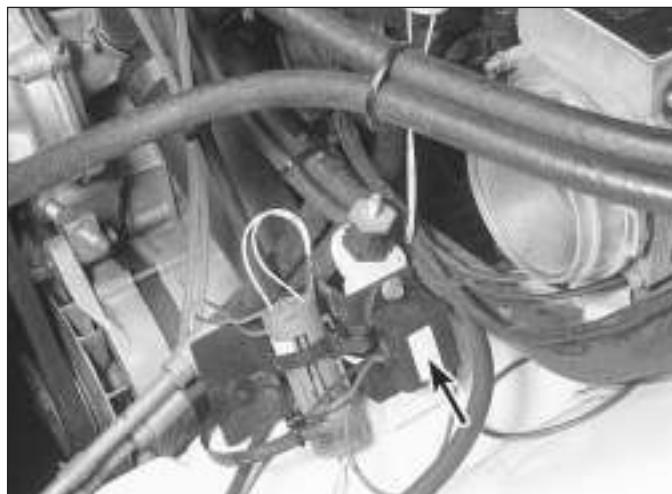
11.9 The load dump module is located on the bulkhead next to the MAF sensor
