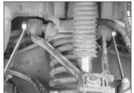
7.5 To detach the upper control arm from the crossmember, remove the nut (at the rear) and pull the bolt out from the front; note the fitted order of the spacer washers
