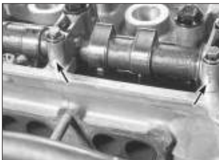
10.11a Each of the camshaft bearing caps are stamped with I (intake) or E (exhaust) and a number (arrowed)
