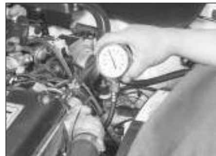
2.4b The oil pressure can be checked by removing the sender unit and refitting a pressure gauge in its place
