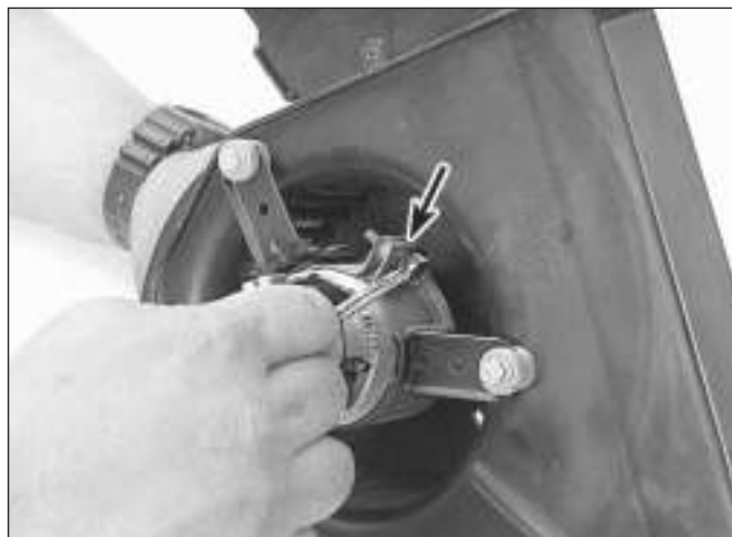
10.11b Loosen the clamp bolt (arrowed) on the motor bracket and then pull the motor and fan out as an assembly
