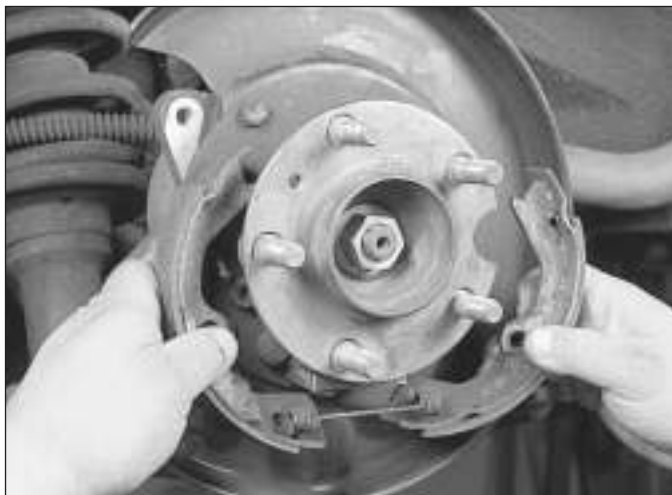
12.5g Pull the shoes apart and remove them with the lower spring attached as shown, then disengage the lower return spring from both shoes
