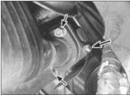
6.3 Remove nuts (small arrows) retaining the exhaust pipe to the manifold flanges; two for each pipe - larger arrow indicates one heat shield bolt accessible from below
