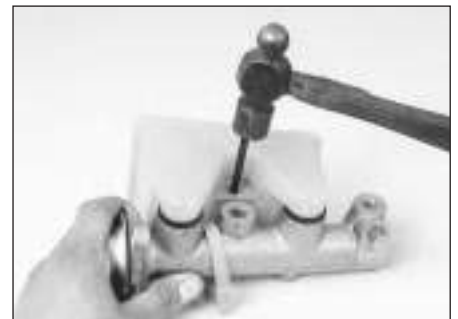
6.7v . . . and tap it into place
