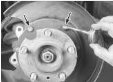
12.5i Lubricate the six friction points (two arrowed) on the backing plate with high-temperature brake grease
