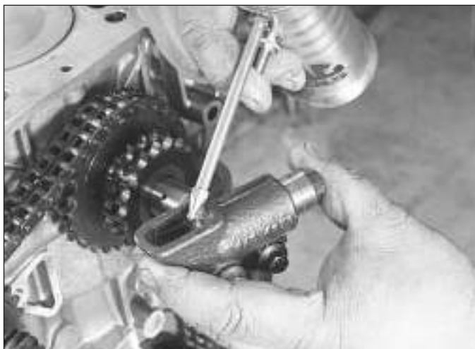
8.23a Add oil to the reservoir in the lower tensioner . . .
