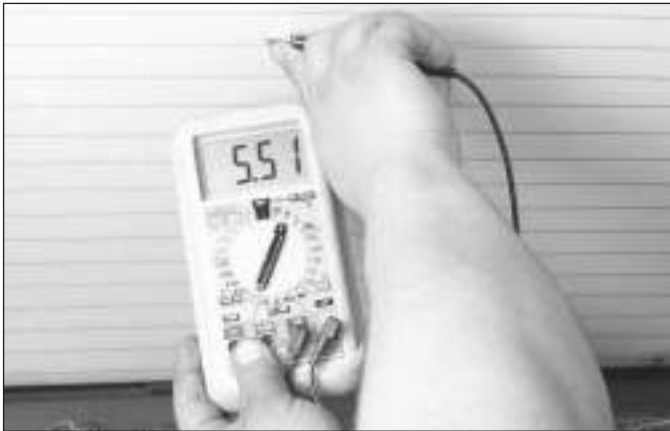
16.5 To determine if a heating element has broken, check the voltage at the centre of each element. If the voltage is 6-volts, the element is unbroken; if the voltage is 12-volts, the element is broken between the centre and the positive end. If there is no voltage, the element is broken between the centre and earth
