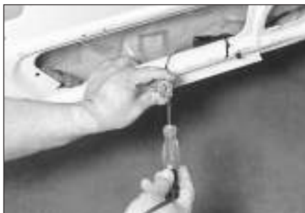
25.6 Check for voltage at the lock solenoid while the lock switch is operated
