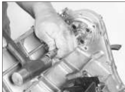
9.11 Tap the seal squarely into the bore with a socket until the seal is flush with the housing, then remove the plastic fitting sleeve
