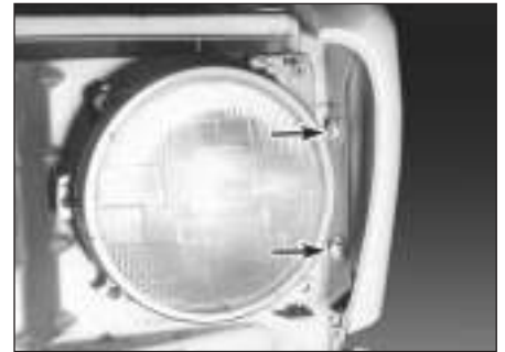
15.7a Detach the wing retaining bolts (arrowed) at the front of the wing
