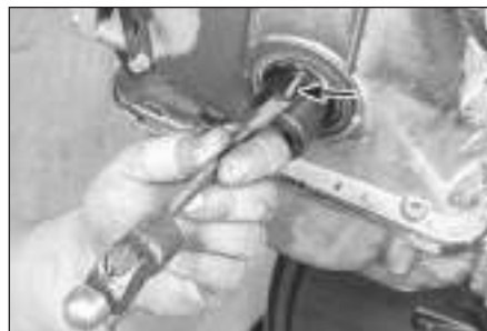
7.7 Carefully tap one end the Woodruff key up and out from the crankshaft keyway, then grasp it with a pair of locking pliers and pull it the rest of the way out - be careful not to damage the key or keyway
