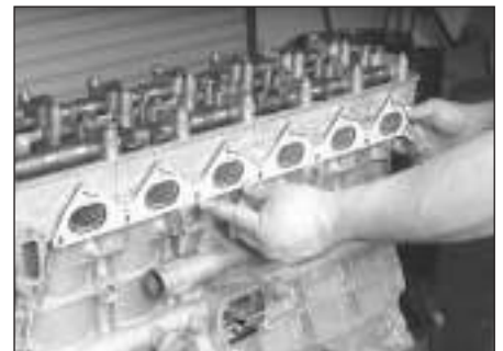
5.9 Refit the new intake manifold gasket over the studs (arrowed) refit the manifold
