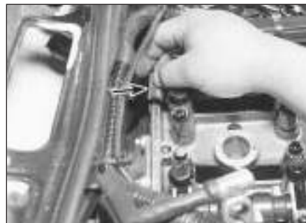
4.6 Apply RTV sealant to the half-circle plugs and insert them into the cylinder head before refitting the valve cover
