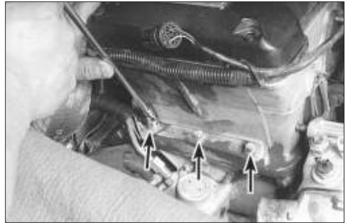
11.11 Remove the bolts (arrowed) securing the cylinder head to the front cover
