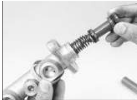
6.7n Apply a coat of clean brake fluid to the primary piston and refit it into the bore
