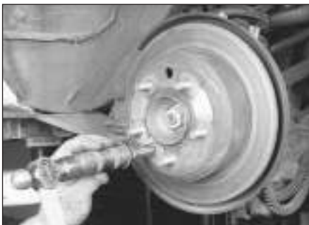
5.7a Using an impact driver, if necessary, remove the disc retaining screw, then remove the disc from the hub
