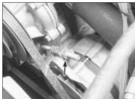
21.6a To adjust the alternator/power steering drivebelt, loosen the outer locknut (arrowed) and the alternator pivot bolt - turn the inner locknut anti-clockwise to loosen or clockwise to tighten the belt
