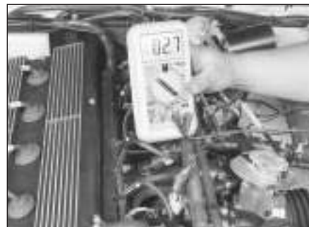
12.9 Using an ohmmeter, measure the resistance across both terminals of the injector
