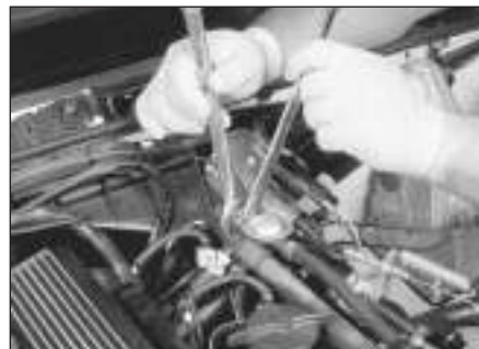
3.6a Remove the fuel line from the fuel pulsation damper . . .
