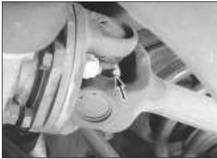
14.6 Grease fittings for the rear driveshafts are located in the centre on each U-joint
