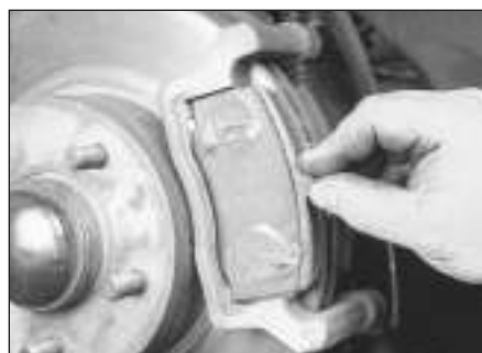
3.5n Refit the outer pad
