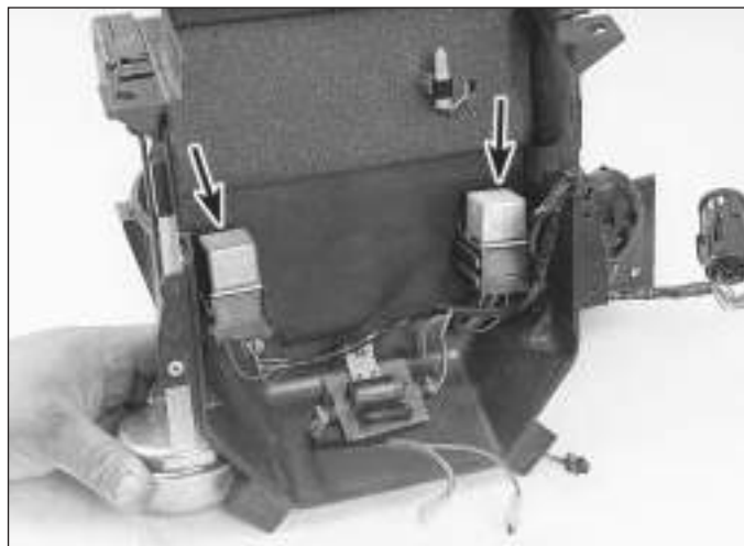
10.12 Inside the blower case are the blower and isolation relays (arrowed) - while the case is apart, test these relays for proper operation
