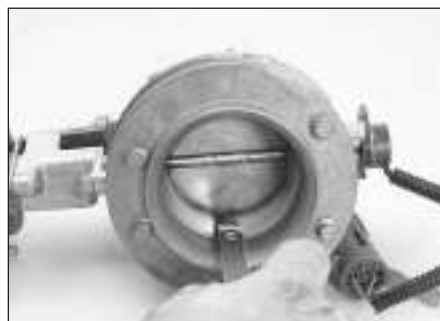
13.19 Measure clearance between the butterfly valve and the throttle body
