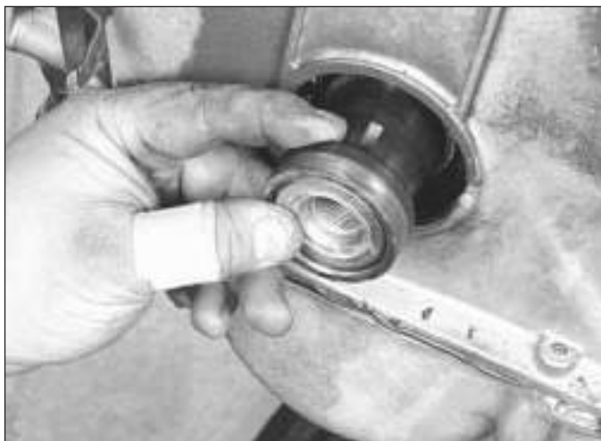
7.9 Remove the spacer from the end of the crankshaft and clean it thoroughly
