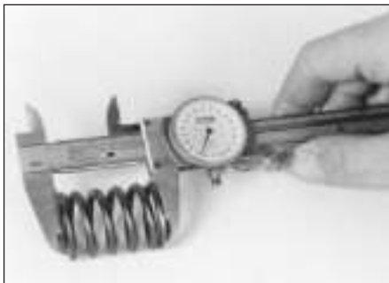
10.18 Measure the free length of each valve spring with a dial or vernier caliper
