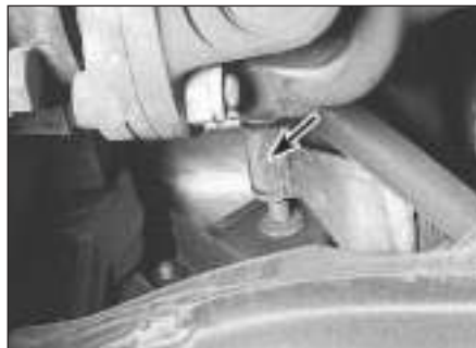
14.1a The rear tailpipe section is fastened to the chassis with a special rubber mount (arrowed) that pivots with road movement. Check for deterioration and alignment
