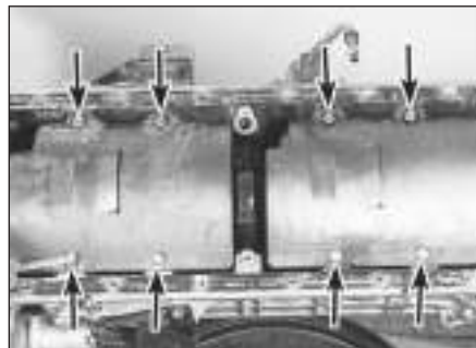
13.2 Remove the screws (arrowed) and remove the front and rear baffle plates
