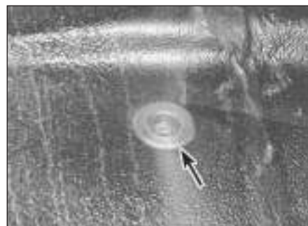
13.16 This drain hose (arrowed) from the heater/air conditioning unit should be kept clear to allow drainage of condensation
