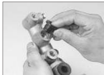
6.7c Remove the grommets, noting the position of each one
