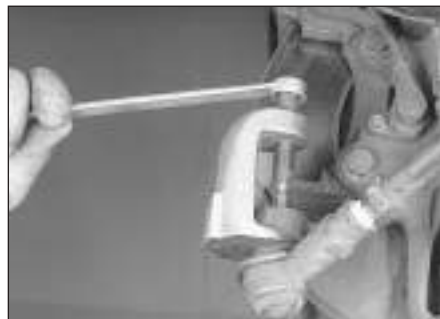
15.3 Loosen the ball stud nut, fit a small puller and pop the ball stud loose from the steering knuckle
