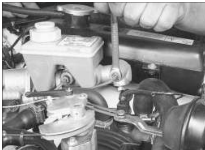
6.5 Loosen the hydraulic brake line fittings with a flare-nut spanner to protect the corners of the nuts
