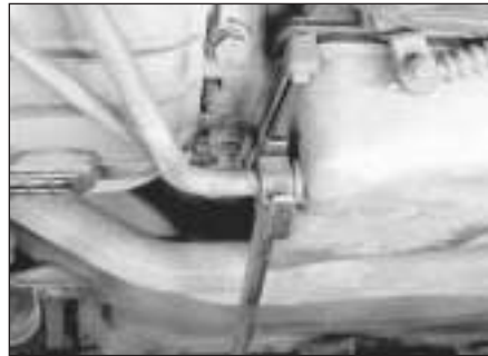
26.6a Unscrew the dipstick tube collar
