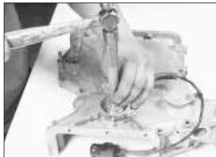
8.28b Drive the new seal in with a seal-driver or socket, to the same depth as the original seal
