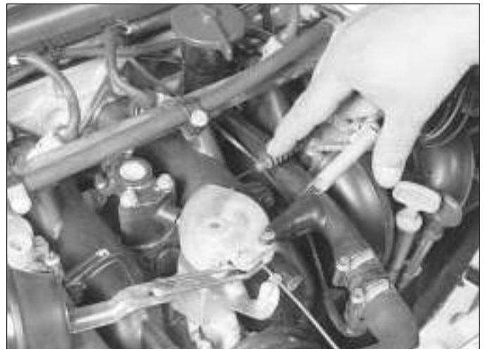
10.9 Make sure the throttle closes completely and there is a slight amount of flex in the cable
