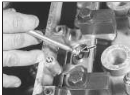
10.18 The valve adjustment shims (arrowed) fit into a pocket in the valve spring retainer - use a magnet to remove the shims and keep them with their respective lifters
