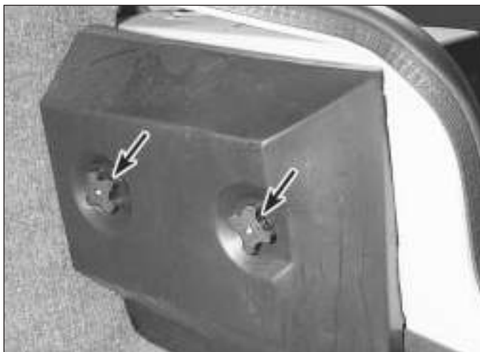
21.4 The Rear direction indicator, brake, tail and reversing light bulbs are accessible from the boot compartment after removing the plastic knobs (arrowed) securing the bulb housing covers
