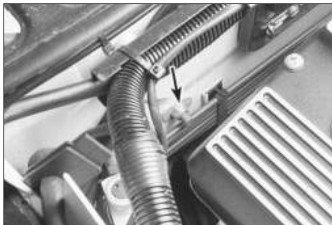
17.4 Remove the housing retaining nut (arrowed) on the engine side of the bulkhead, near the expansion valve - another nut is on the right, near the heater core pipes
