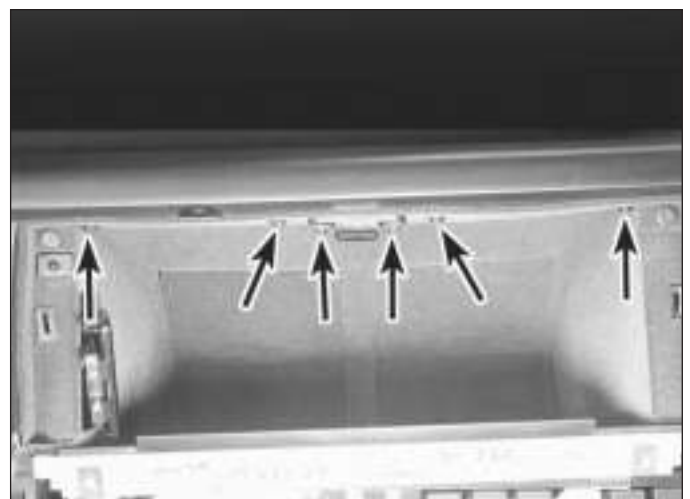
26.11 Remove the screws along the top edge (arrowed), pull the glove box out and remove the lamp assembly
