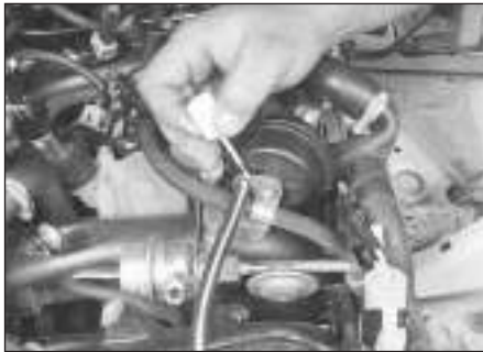
5.3 The various hoses should be marked to ensure correct refitting
