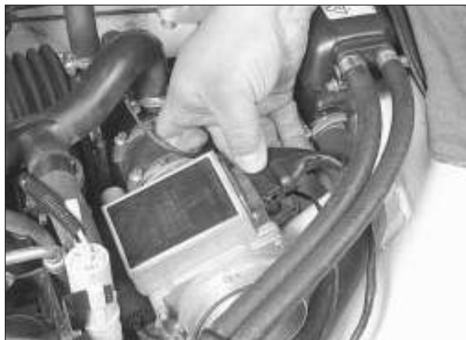
13.7 Push up on the clip and remove the harness connector from the MAF sensor
