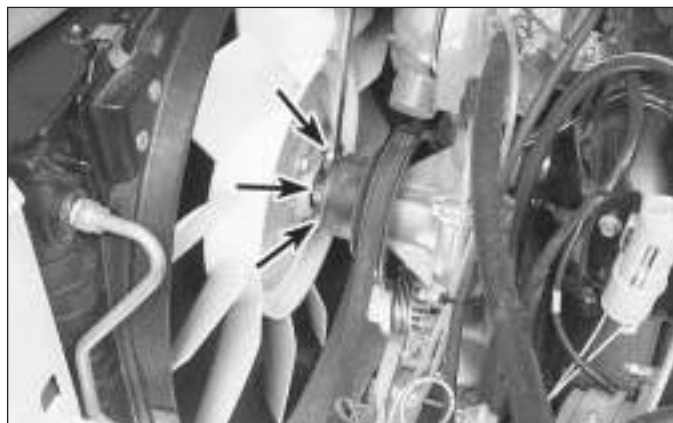
4.8 Remove the four nuts (arrows indicate three shown here) holding the fan/clutch assembly to the front of the water pump
