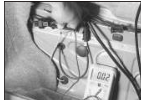
3.4b Check for battery voltage to the fuel pump on the harness connector near the fuel tank on models with in-tank fuel pumps
