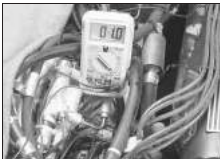
8.3a To check the primary resistance of the coil, measure the resistance between the positive and the negative terminals
