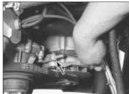
12.3 Loosen the lock bolt and back-off the adjustment bolt (arrowed) to remove the drivebelt
