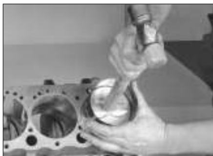
25.11 The piston can be driven (gently) into the cylinder bore with the end of a wooden or plastic hammer handle
