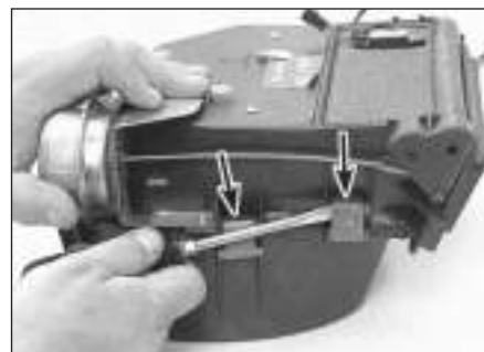
10.10 Remove the five clips (two shown here with arrows) and one screw holding the halves of the housing together
