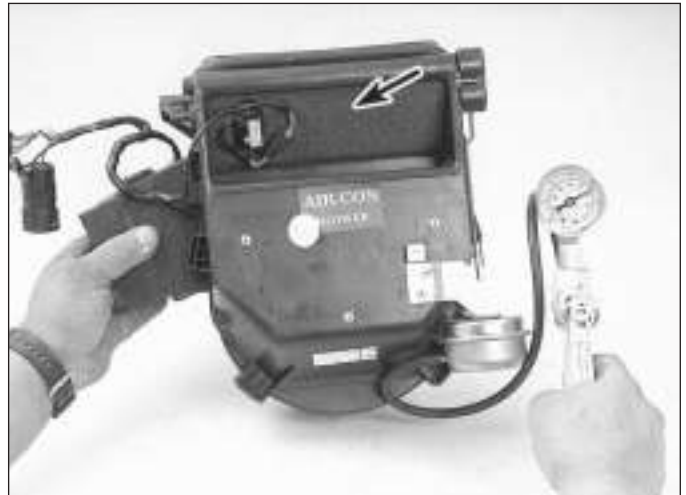
12.11 Check the operation of the vacuum servo motors; in this case, vacuum is applied to the servo on the right blower case - the flapper door (arrowed) should operate
