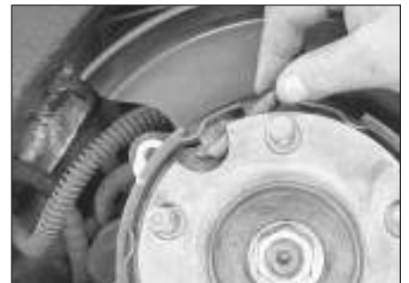
12.5p Hook the upper return spring into the front shoe . . .
