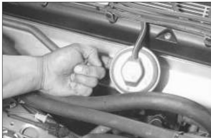
6.5 Use a fingertip to move the diaphragm inside the EGR valve
