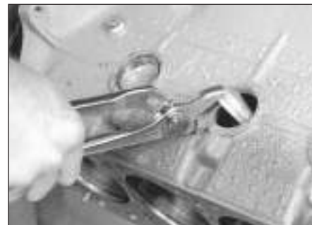
15.1b Pull the core plugs from the engine block with pliers
