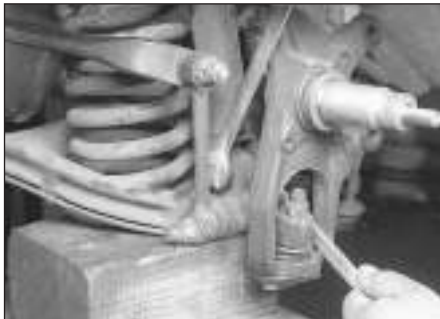
4.3 To disconnect the lower end of the shock absorber from the lower control arm, remove this nut and bolt
