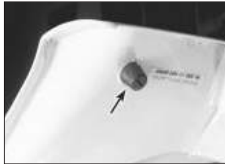
16.10 Turn the bump stops in or out so the boot lid is flush with the rear wings when in the closed position
