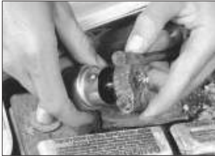
6.7a Remove all the corrosion from the cable clamps (the inside of the clamp is tapered to match the taper on the post, so don't remove too much material)
