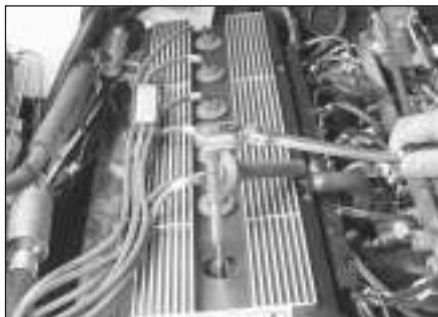
4.8 Use a spark plug socket with a long extension to unscrew the spark plugs
