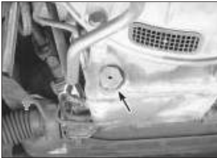
3.7 The oil drain plug (arrowed) is located at the rear of the sump - use a ring spanner or socket to remove it
