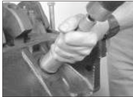
15.10 A large socket on an extension can be used to drive the new core plugs into the bores
