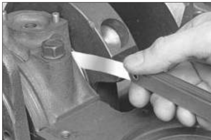
14.3 Checking crankshaft endplay with a feeler gauge
