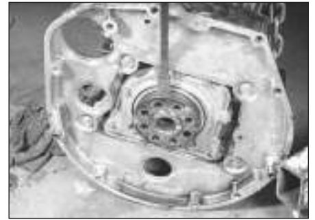
14.4 Pry off the driveplate spacer - if a driveplate is replaced, the spacer should be replaced also
