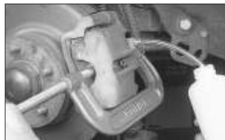
3.5b Attach a hose to the bleed screw, open the bleed screw slightly and depress the piston into the caliper. Tighten the bleed screw when the piston bottoms
