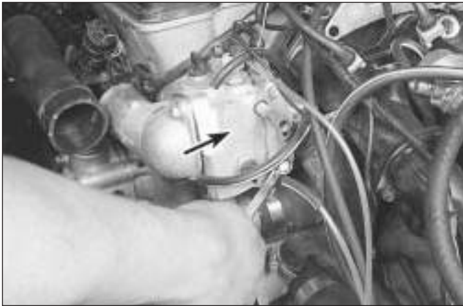
11.10 Disconnect the hoses and remove the bolts to separate the coolant housing (arrowed) from the cylinder head
