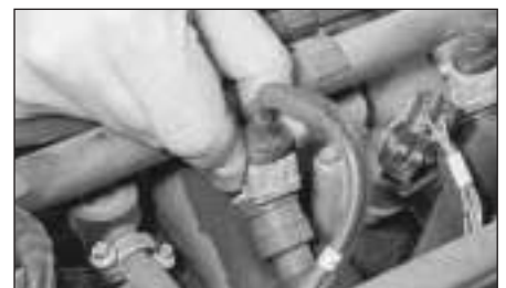
D Check that the wiring connectors are securely connected to the injectors and various fuel system sensors and switches.
