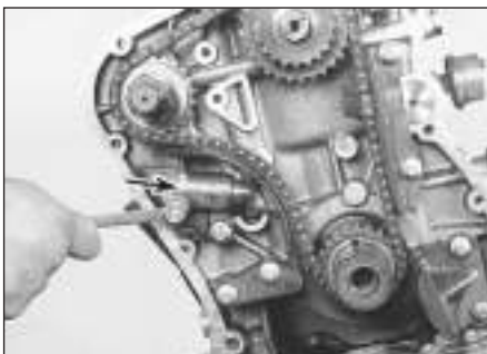
8.13 Remove the two bolts and remove the lower timing chain tensioner (arrowed)
