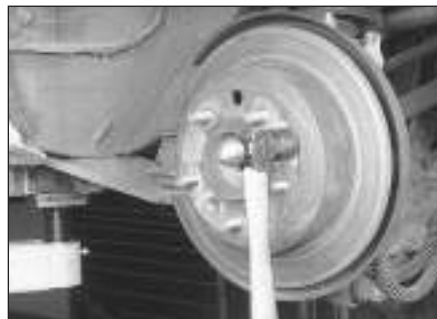
5.7b If the disc is stuck to the hub, give it a few sharp raps with a hammer
