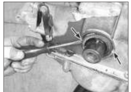
7.8 Remove the crankshaft seal with a screwdriver or seal puller - there are two slots (arrowed) in the cover which allow you to pry behind the seal
