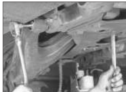
13.6 Hold the pivot bolt and unscrew the nut
