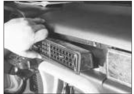
24.7 After removing the centre trim panel, detach the air conditioning duct
