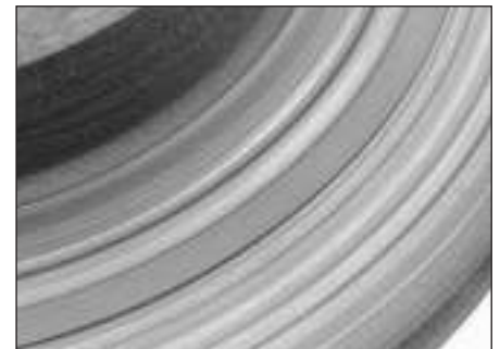
5.3 The brake pads on this vehicle were obviously neglected, as they wore down to the rivets and cut deep grooves into the disc - this disc must be replaced
