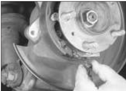
12.5l Hook the lower return spring into its hole in the front shoe . . .
