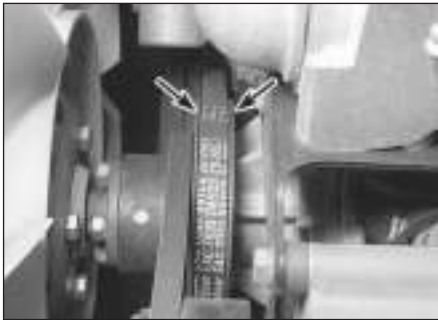
21.11 When refitting ribbed (serpentine) drivebelts, make sure the belt is centred between the pulley edges (arrowed) - it must not overlap either edge of the pulley
