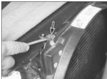
4.10 Pry out the two clips (arrow indicates the left one) at the top of the fan shroud and lift out the shroud
