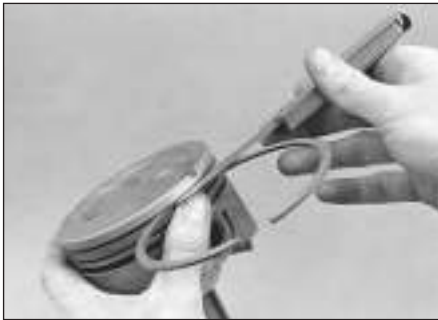
18.10 Check the ring groove clearance with a feeler gauge at several points around the groove
