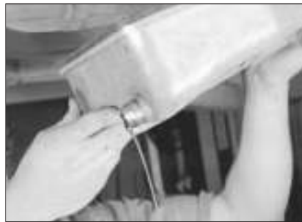
26.8 Lower the sump pan from the transmission
