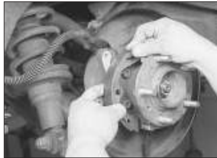
12.5j Place the front shoe in position, insert the pin through the backing plate and the shoe . . .
