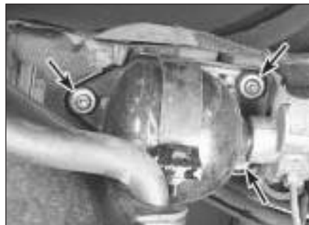
7.4 Remove these three Torx screws (arrowed) and move the accumulator assembly to the side a little to provide clearance for pulling out the pivot bolt
