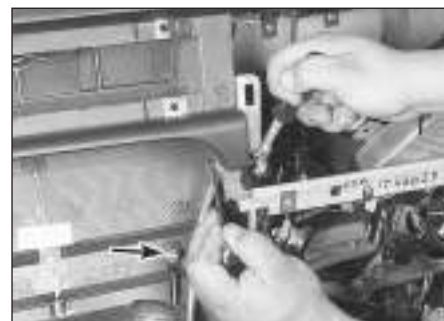
17.9b Black case-support rods are held with nuts (arrowed), the gold dash-support rods are retained by a bolt/nut to the dash
