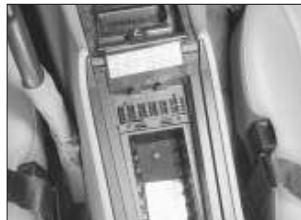
3.1c A third fusebox is located in the centre console glove box
