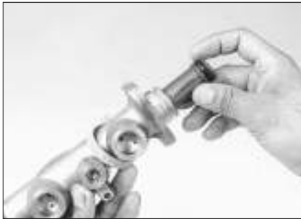
6.7m Apply some clean brake fluid to the secondary piston and refit it with the slot oriented with the stopper pin hole, so that the stopper pin will go through the slot
