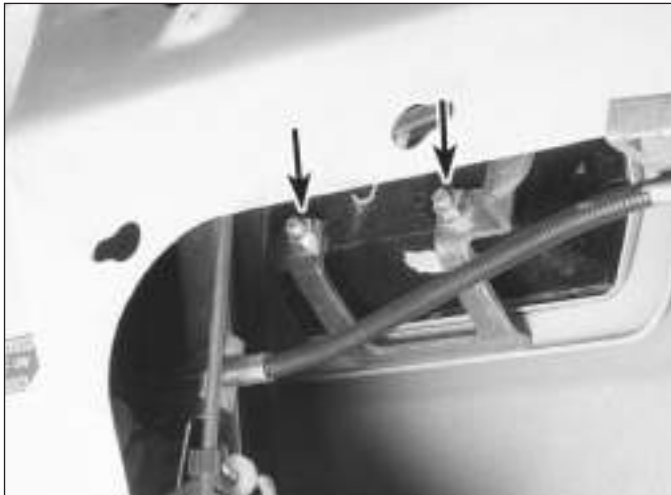
20.7 The outside handle retaining nuts (arrowed) can be reached through the access hole in the door
