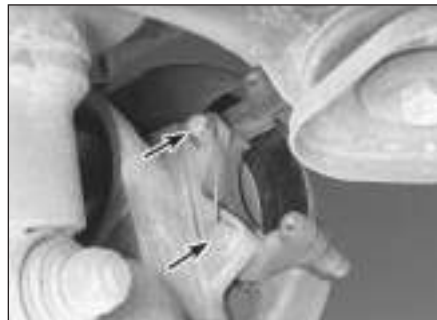
5.6a Before you can remove the caliper mounting bracket bolts (arrowed) and the bracket, you'll have to cut the safety wire between them with a pair of diagonal cutters (rear bracket shown)
