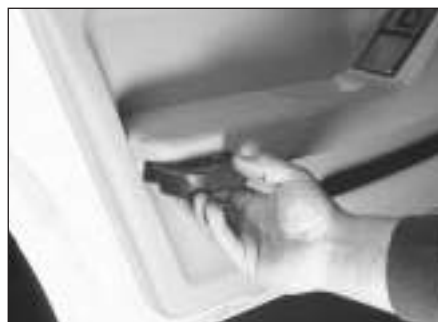
18.7a Prise out the courtesy lamp lens
