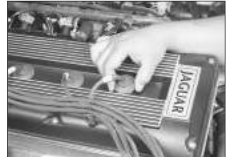
4.6 When removing the spark plug leads, grasp only the boot and use a twisting/pulling motion
