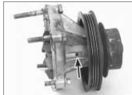
7.3 Check the weep hole (arrowed) for signs of leakage (pump removed for clarity) - grey discoloration is normal, large brown stains indicates seal failure
