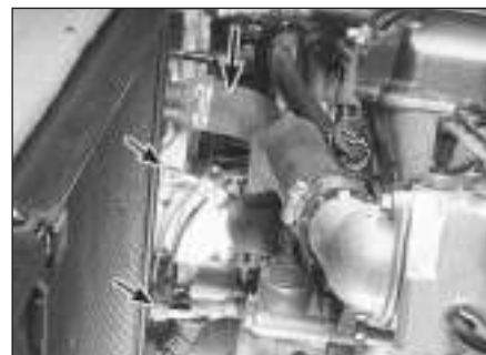
5.5b Disconnect the power steering cooler lines (small arrows) at the right side of the radiator, and the upper radiator hose (large arrow)
