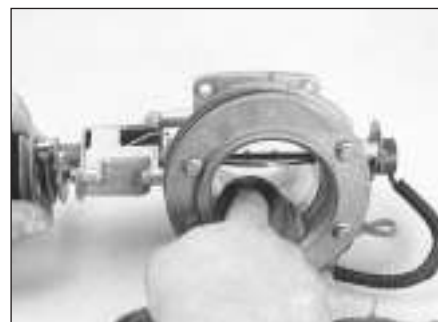
13.18 The area inside the throttle body near the throttle plate suffers from sludge build-up because the PCV hose vents crankcase vapour into the intake duct
