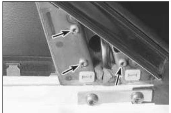
23.4 Disconnect the electrical connector, then detach the three mirror retaining screws and remove the mirror from the vehicle
