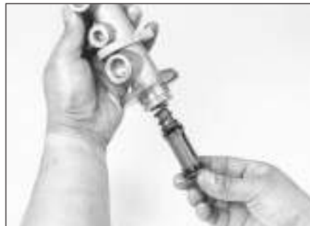
6.7h Remove the secondary piston
