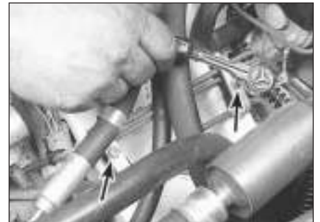
10.10c . . . then remove these bracket screws (arrowed), the brackets and the forward section of hydraulic line
