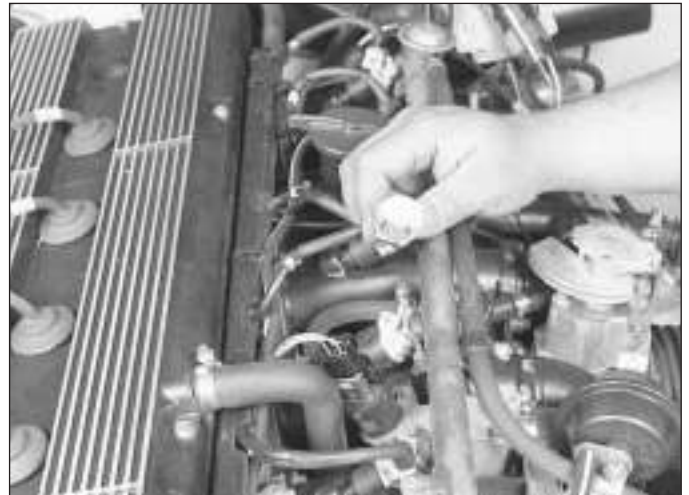
12.8 Refit the "noid" light into the fuel injector electrical connector and check to see that it blinks with the engine running
