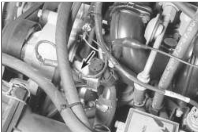
5.6 Location of the AIR diverter valve on a 1992 model - check the hoses for cracking and the electrical connector for security
