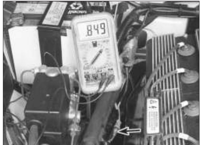
4.15 Refit a pin into the backside of the oxygen sensor connector into the correct terminal and check for a millivolt output signal generated by the sensor as it warms up. The SIGNAL wire is easily recognised by the rubber sheath covering the terminal (arrowed)
