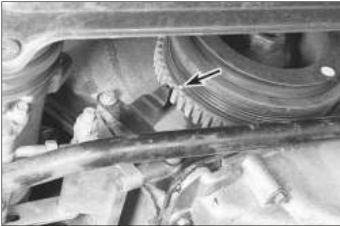
3.8 Align the mark on the crankshaft sensor ring (arrowed) with the bottom edge of the pointer on the front cover
