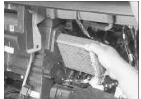
11.8 Pull the heater core out to the right
