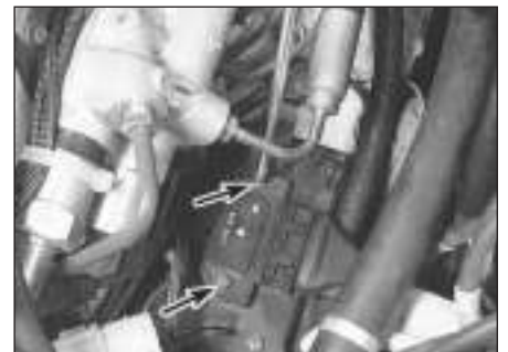
7.5 Remove the amplifier mountings screws (arrowed) and lift the unit from the engine compartment
