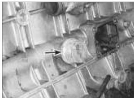
2.4a The oil pressure sender unit (arrowed) is located in the right front corner of the engine block, near the oil filter
