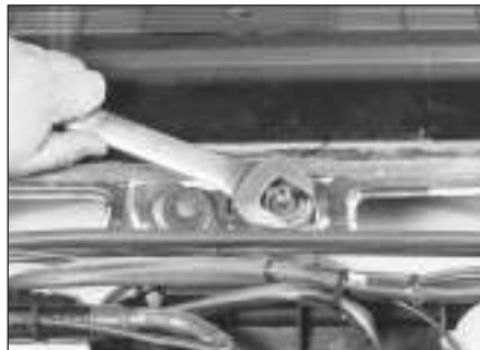
15.3 Use a spanner or socket to remove the drive spindle retaining nut
