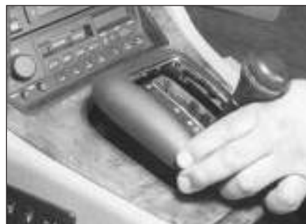
24.2 Carefully prise out the gear selector trim bezel
