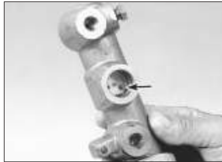
6.7e Locate the stopper pin (arrowed) inside the forward grommet hole . . .
