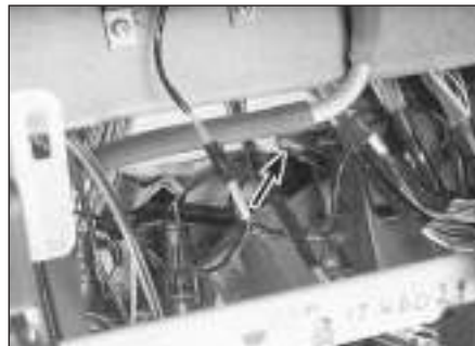
10.5 Two bolts (arrow indicates the left bolt) hold the top of the blower housing to the cowl
