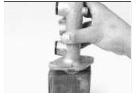
6.7i If the secondary piston is stuck, rap the master cylinder on a wood block to dislodge it
