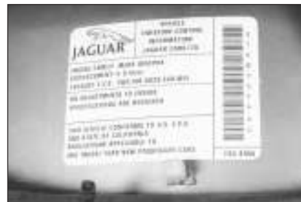
1.6a The Vehicle Emissions Control Information (VECI) label shows the types of emission control systems installed, engine information, etc (1992 model shown)
