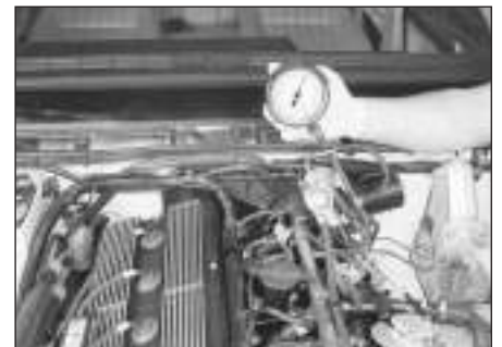
3.6b . . . then refit the fuel pressure gauge between the fuel rail and the fuel pressure damper using a T-fitting
