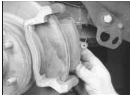
3.5g Remove the inner brake pad
