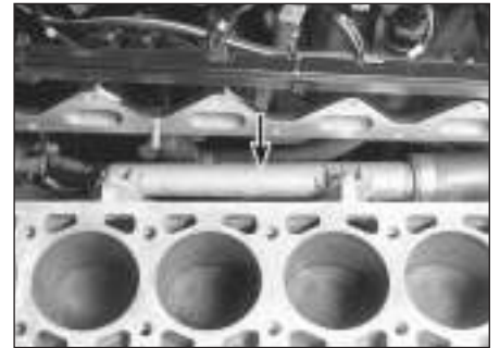
8.8b The water pipe (arrowed) may need new gaskets where it meets the block - the pipe is best accessed from below or with the intake manifold unbolted
