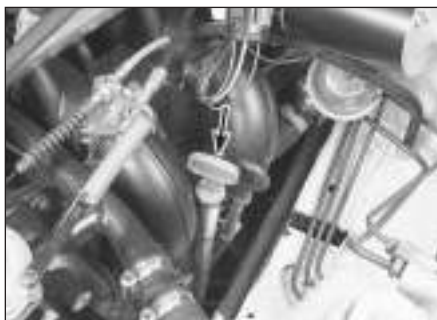
8.4a The automatic transmission dipstick (arrowed) is located in a tube which extends forward from the transmission
