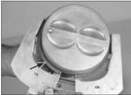
22.12 Refit the compression rings with a ring expander - the mark must face up
