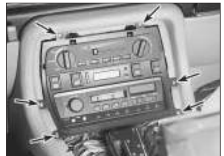
12.3a Remove these six screws (arrowed) to release the control panel/radio assembly from the console
