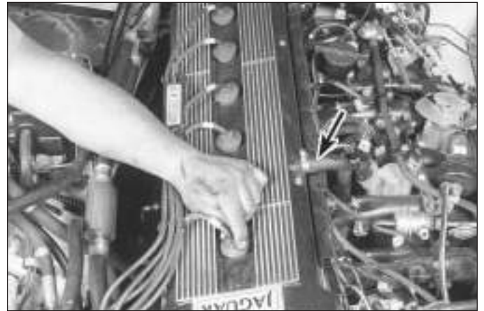
4.2 Disconnect the PCV hose (arrowed) from the valve cover, then pull the spark plug leads out by their boots, not the leads
