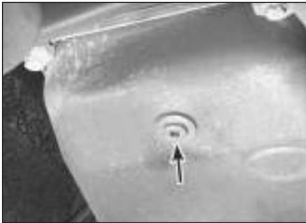
26.5 Using an Allen spanner remove the drain plug located in the bottom of the transmission sump pan
