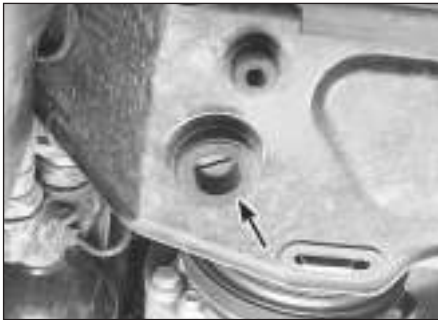
30.4 The radiator drain fitting (arrowed) located at the bottom of the radiator
