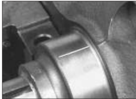
23.10 Lay the Plastigauge strips on the main bearing journals, parallel to the crankshaft centreline
