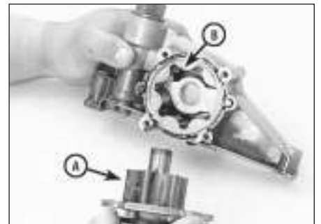
13.7b Remove the outer rotor (A) and inner rotor (B)
