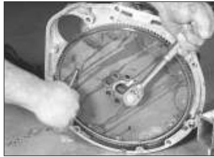
14.3 Use a screwdriver to secure the flywheel while the bolts are removed
