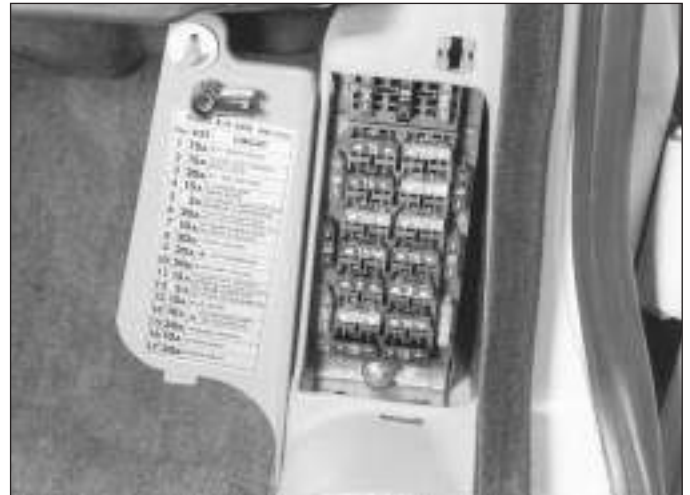
3.1b The right side fusebox is located in the driver's side kick panel, behind the fuse panel cover
