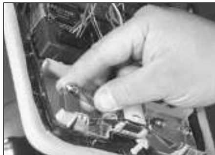
21.9 The interior light bulbs can be accessed after lowering the overhead console
