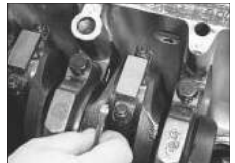
13.3 Check the connecting rod side clearance with a feeler gauge as shown
