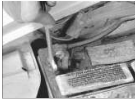
6.6b Removing a cable from the battery post with a spanner - sometimes special battery pliers are required for this if corrosion has damaged the nut hex
