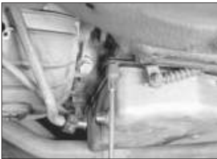
26.7 Use a socket and extension to remove the transmission sump pan bolts and brackets
