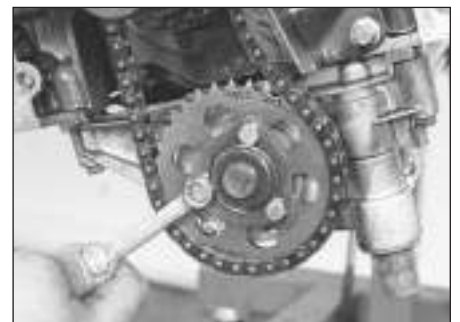
13.4 Pry back the locking tabs and remove the three bolts retaining the oil pump drive sprocket to the pump
