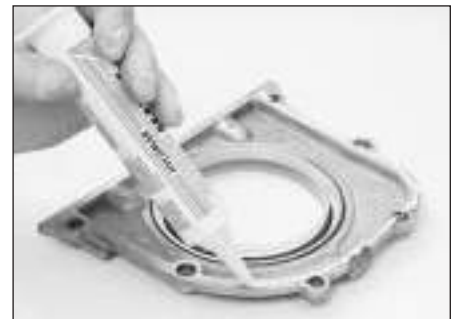
15.5 Apply RTV sealant to the sealing surface
