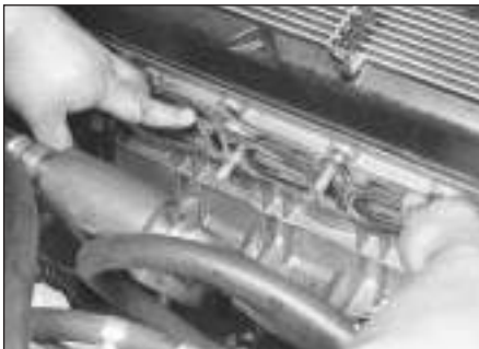
6.8 Refit new gaskets in position over the studs with the markings facing out
