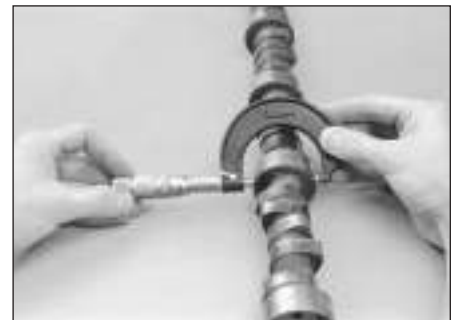
10.20 Measure the bearing journals with a micrometer to check diameter - measure at several places around the journal to check for taper or out-of-round
