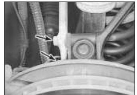
5.8 Remove the bolts and shims from the upper balljoint; be sure to put the shims back when refitting the new balljoint
