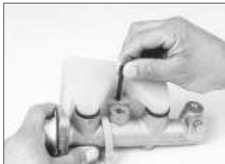
6.7u Refit the reservoir roll pin . . .
