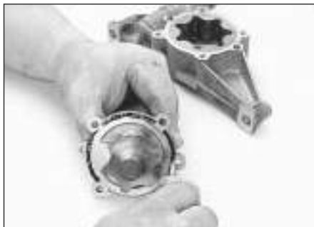
13.14 Apply a thin coat anaerobic sealant (Loctite 510 or 518) to the pump cover sealing surface
