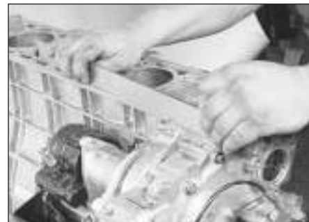
8.29 Bolt the front cover on hand tight, use a straightedge to make sure the cover's top surface is level with the top of the engine block, then tighten the cover bolts
