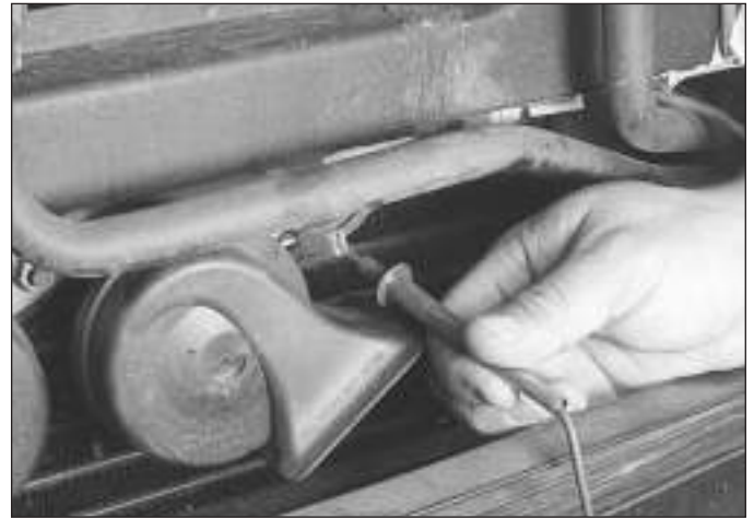
20.3 Check for power at the horn terminal with the horn button depressed
