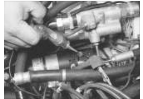
6.11 Refit the LED test light to the coil negative (-) terminal, crank the engine over and observe the light flash in response to the trigger signal from the computer
