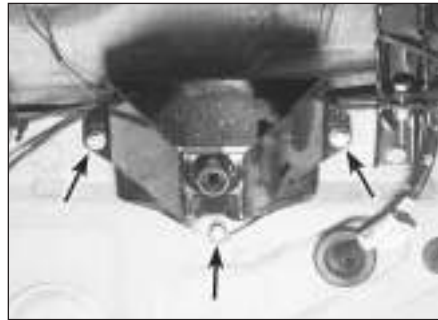
7.8 Remove the bolts (arrowed) from the spare tyre bracket and lift out the assembly
