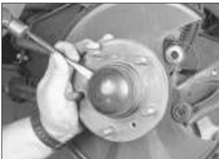
22.6 Dislodge the dust cap by working around the outer circumference with a hammer and chisel
