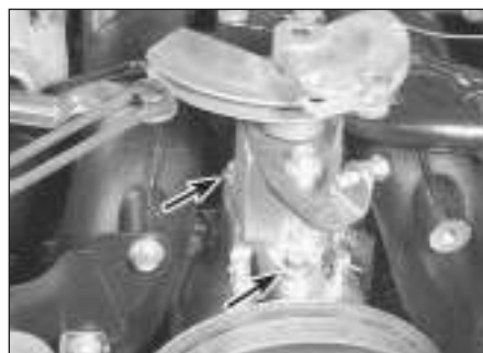
13.9 Remove the bellcrank assembly bolts (arrowed) and separate it from the throttle body
