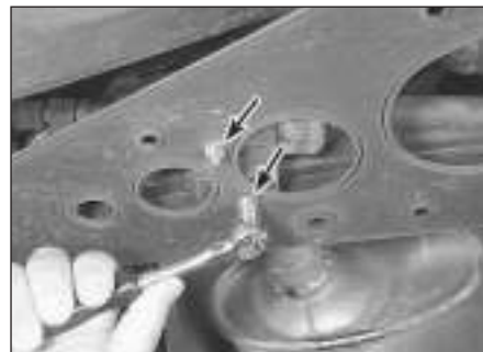
4.6 Remove the fuel pump mounting nuts (arrowed) and slide the fuel pump out of the rubber casing (1989 model shown)
