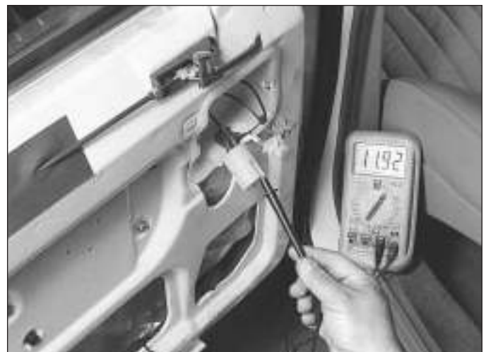
24.12 If no voltage is present at the motor with the switch depressed, check for voltage at the switch
