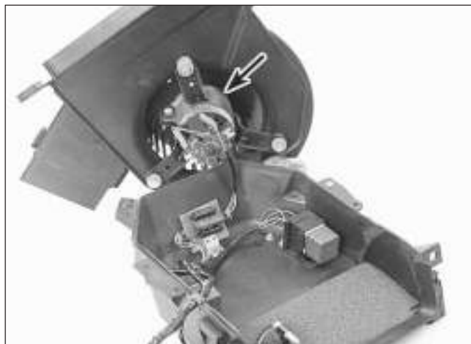
10.11a Separate the housing halves - the blower motor (arrowed) is attached to a plastic plate sandwiched between the two housing halves
