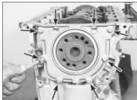
15.2 Remove the bolts (arrowed) and the crankshaft rear oil seal retainer from the back of the engine block
