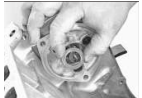
9.10 Refit the washer before replacing the snap-ring
