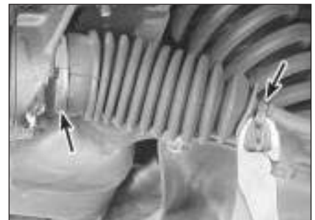
16.2 Cut off the boot clamps (arrowed) and slide the boot off the steering gear
