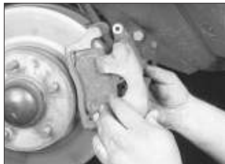
3.5d Remove the caliper . . .
