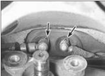
7.9d Remove the clips (arrowed) that retain the fuel lines to the fuel tank using needle-nose pliers
