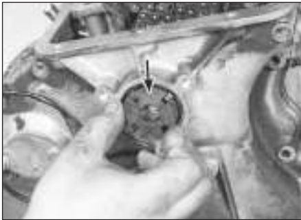
8.9a Pull the hydraulic pump coupling disc (arrowed) off the drive coupling . . .
