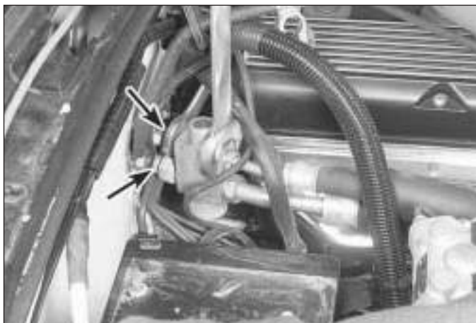
17.2 Use two spanners when disconnecting the air conditioning lines (arrowed) at the bulkhead, on the backside of the expansion valve - one spanner holds the body of the expansion valve
