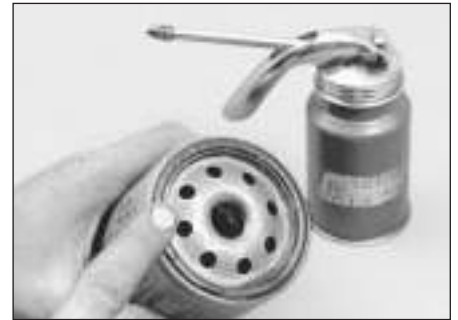
3.15 Lubricate the oil filter gasket with clean engine oil before refitting the filter
