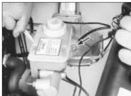
6.6 Remove the two master cylinder mounting nuts
