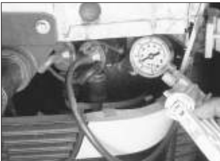
7.12 Remove the front spoiler to gain access to the purge control valve (see Chapter 11). Apply vacuum to the valve and make sure the valve holds vacuum
