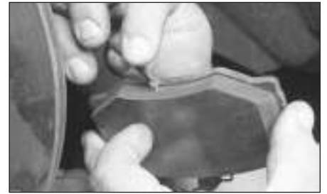
3.5h Pull out the wear sensor, trace the sensor lead back to its plug, detach the lead from the suspension, and discard it
