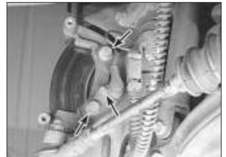
5.6b On front caliper brackets, remove the ABS wheel speed sensor bolt (centre arrow) and pull out the sensor before removing the bracket bolts (upper and lower arrows) and bracket
