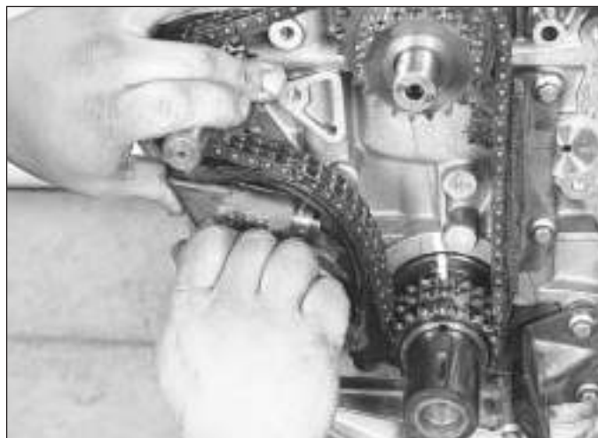
8.23b . . . and refit the tensioner against the guide - after it's installed, push the tensioner guide back and forth a few times to prime the tensioner
