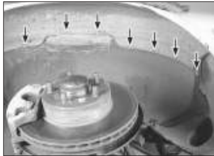
15.4 Remove the bolts (arrowed) securing the inner wing splash shield
