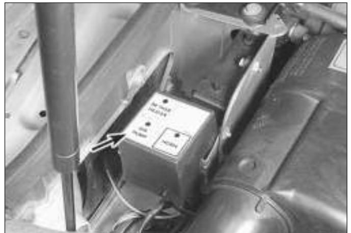
5.5 Location of the AIR pump relay on a 1992 model
