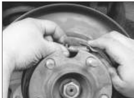
12.5b Back off the star wheel on the adjuster, then disengage the adjuster mechanism from the handbrake shoes
