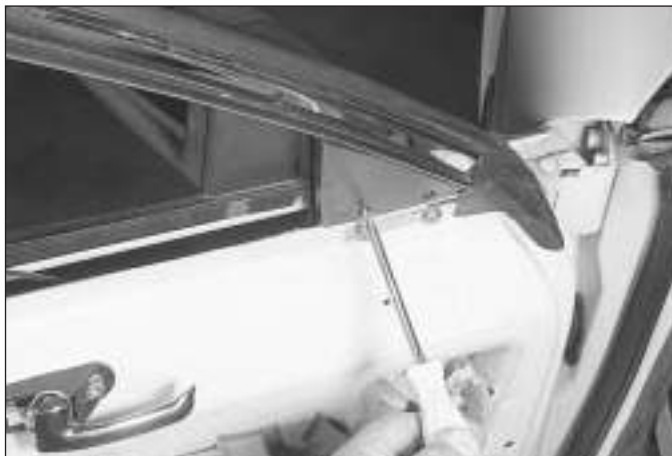
23.2 Remove the trim cover retaining screws
