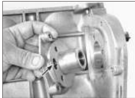
9.9 Refit the auxiliary shaft rear housing with a new gasket, aligning the oil slot (arrowed) with the housing
