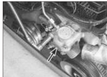
8.7 Unbolt the hydraulic pump (arrowed) from the front cover, without disconnecting the hoses
