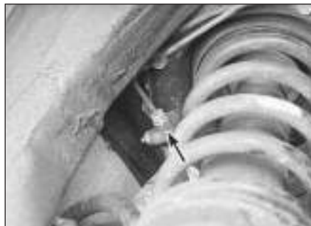
10.2a On a vehicle equipped with self-levelling rear suspension, the valve block (arrowed) for the left rear shock is located just in front of the shock absorber
