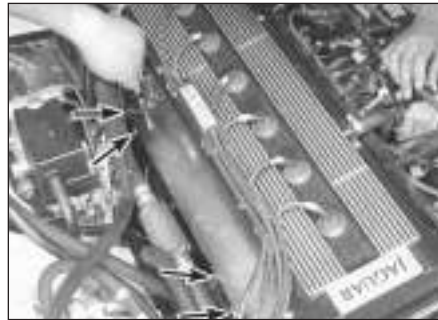
6.4 Remove the upper heat shield bolts (arrowed)
