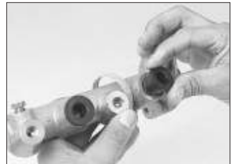
6.7r Refit the grommets
