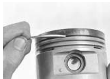
18.4b . . . or a section of a broken ring
