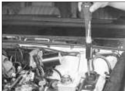
2.4 An inexpensive hydrometer can be used to test the condition of your coolant
