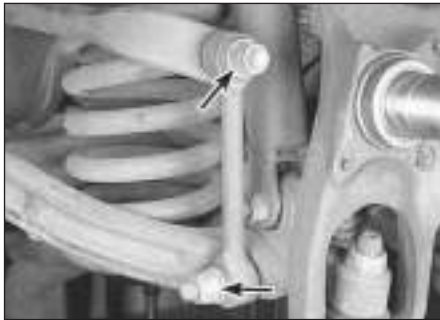
3.3 To disconnect the anti-roll bar from the link, remove the upper nut (arrowed); to disconnect the link from the lower control arm, remove the lower nut (arrowed)
