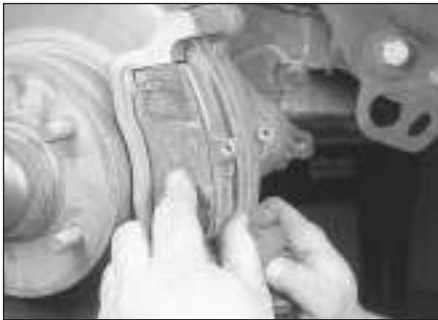
3.5f Remove the outer brake pad
