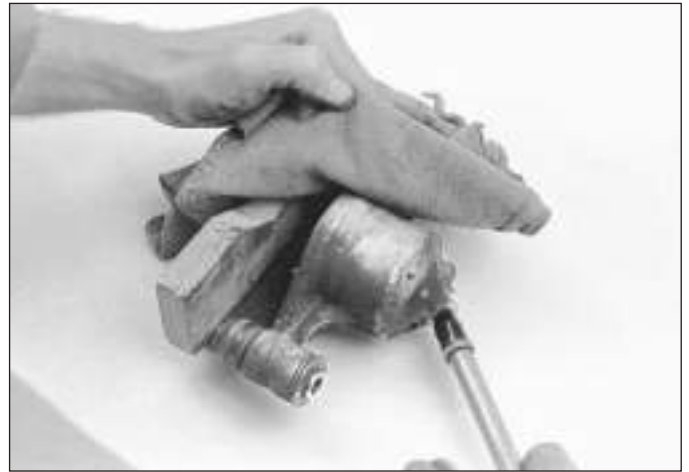
4.5 With the caliper padded to catch the piston, use compressed air to force the piston out of its bore - make sure your fingers are not between the piston and the caliper
