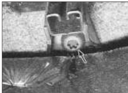
29.2 Use a Torx bit to remove the front seat retaining bolts (arrowed)
