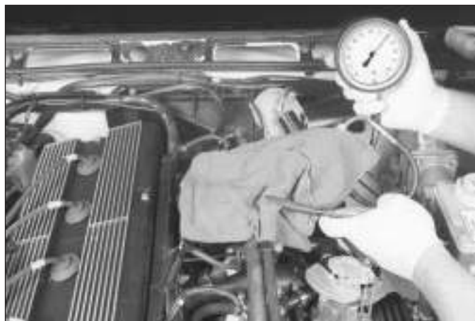
3.12 Using a pair of pliers, squeeze the return line and observe the fuel pressure increase (wrap a rag around the fuel line so you don't damage it)
