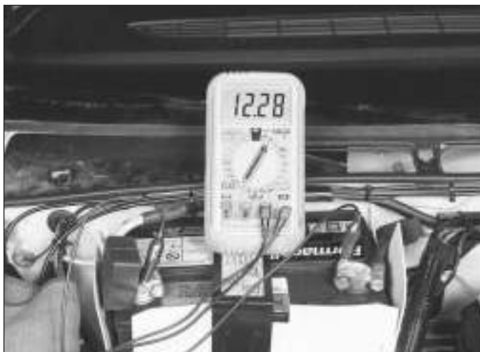
11.2 Connect the probes of a voltmeter to the battery terminals and observe battery voltage with the engine OFF and then with the engine running
