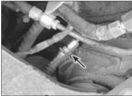
8.3b The connection (arrowed) for the rear hose and line is located right above the mounting bracket for the front corner of the differential crossmember; remove the hose as described in the previous illustration
