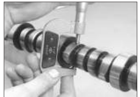
10.21b . . . and subtract the camshaft lobe diameter at its smallest dimension to obtain the lobe lift
