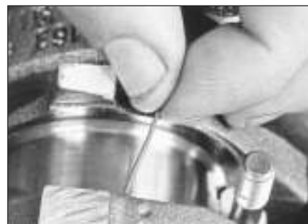
25.13 Lay the Plastigauge strips on each big-end bearing journal, parallel to the crankshaft centreline
