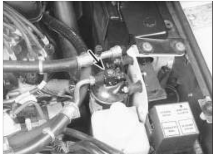
13.11 The sight glass (arrowed) is located on the top of the receiver/drier, to the right of the radiator
