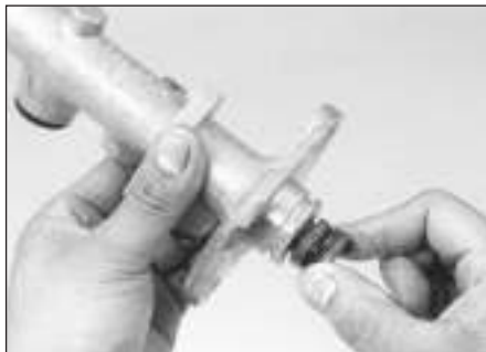
6.7g Remove the primary piston
