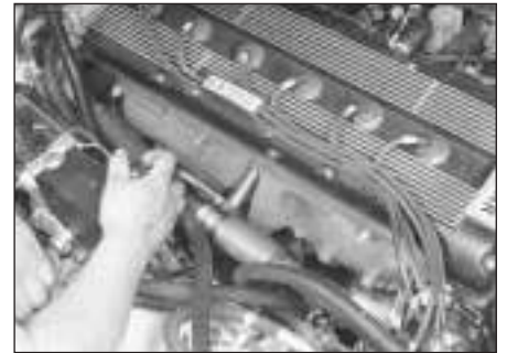
6.6 Remove the bolts and nuts and remove the front and rear exhaust manifolds
