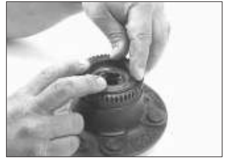
22.19 After refitting the inner wheel bearing into the hub - press the grease seal into place
