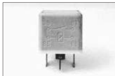
6.3 Most relays are marked on the outside to easily identify the control circuit and power circuits
