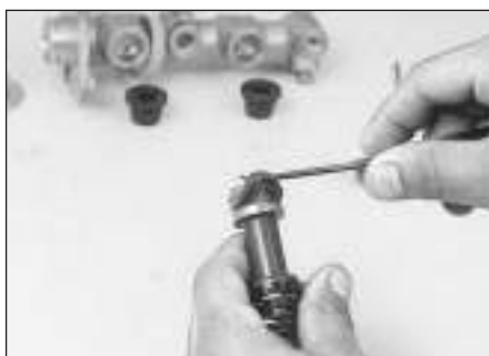
6.7j Remove the seals and cups from the pistons - be very careful not to scratch the piston surface - then wash the secondary piston with clean brake fluid and inspect it; if the secondary piston is damaged, you must renew the master cylinder with a new or rebuilt unit (a new primary piston is included with the rebuild kit)
