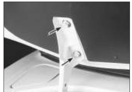
16.4 With the help of an assistant to hold the boot lid, remove the retaining bolts and lift off the boot lid
