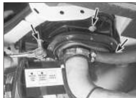
7.7a Remove bolts (arrowed) that retain the fuel filler assembly to the body and slide the assembly down the filler neck of fuel tank
