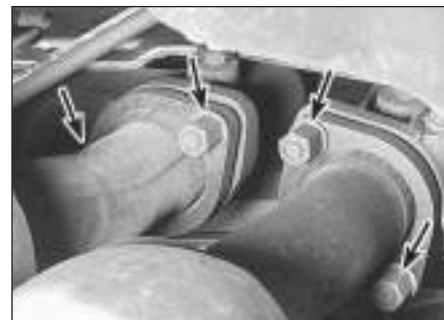
14.4 Use penetrating spray on the exhaust flange nuts before attempting to remove them
