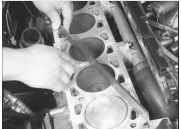
10.13 Check the cylinder head and engine block gasket surfaces for warpage by trying to slip a feeler gauge under a precision straightedge (see the Specifications for the maximum warpage allowed and use a feeler gauge of that thickness) - check both the cylinder head and engine block (shown)
