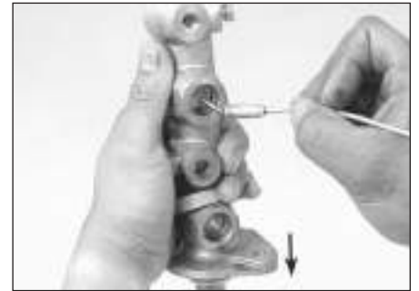
6.7f . . . insert a punch into the pocket of the primary piston, place the master cylinder vertically as shown, push down on the master cylinder to depress the pistons and pull out the stopper pin with a magnet
