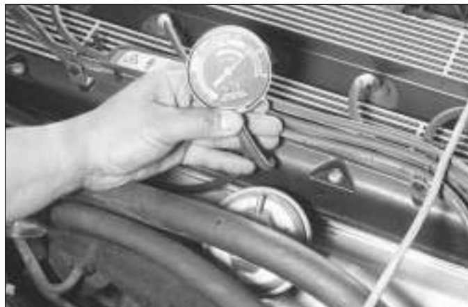
6.6 Check for vacuum to the EGR valve from the throttle body
