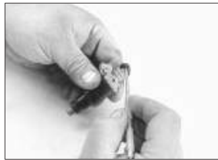
13.38b Pick out the old injector seal but make sure the injector body is not damaged in the process
