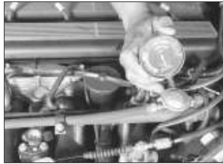
3.4 The vacuum gauge is easily attached to a port on the intake manifold, and can tell a lot about an engine's state of tune
