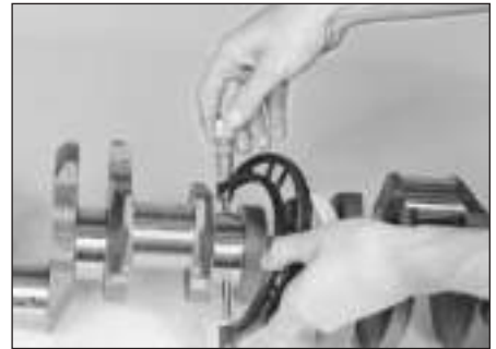
19.5 Measure the diameter of each crankshaft journal at several points to detect taper and out-of-round conditions
