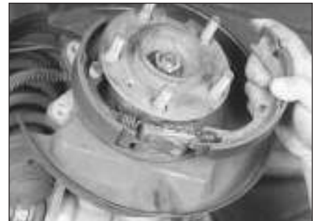
12.5n . . . stretch the spring over the top of the handbrake lever box . . .
