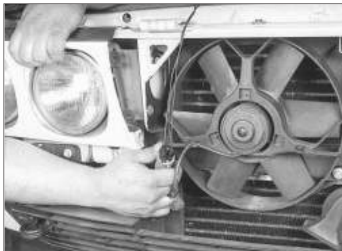
4.17 Disconnect the fan wiring connector and connect jumper wires from there directly to the positive and negative terminals of the battery - the purple wire's terminal should receive the battery power and the black wire's terminal should be earthed
