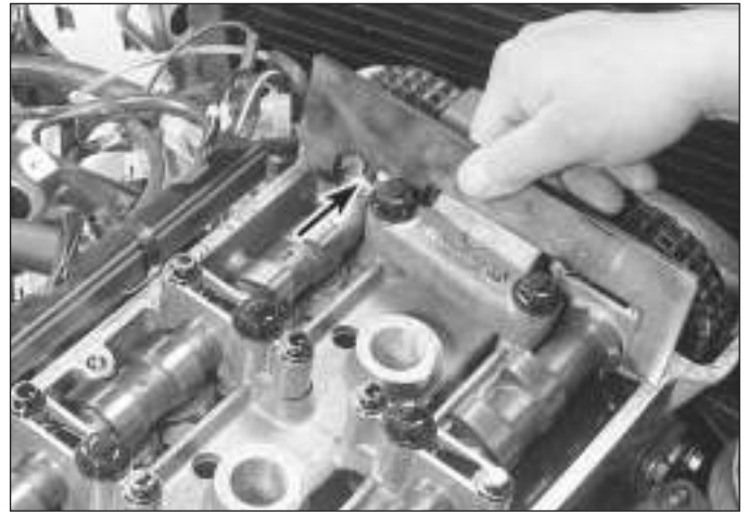
10.5 Position the camshaft alignment tool over each camshaft - the projection on the tool only fits into the slot on the camshafts when they are at TDC - flip the tool over to check the other camshaft
