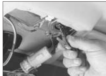
27.9 To close the sunroof manually, insert the T-handle spanner in the motor shaft and rotate it clockwise
