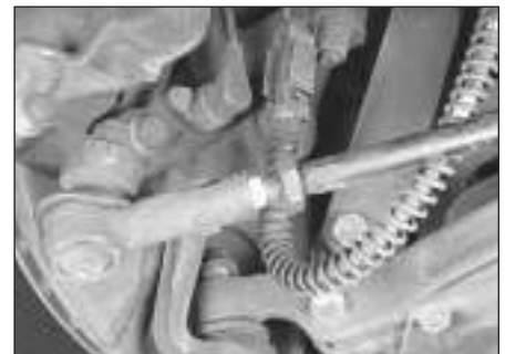
15.2 Back off this locknut and mark the threads to ensure that the new tie-rod end is installed properly
