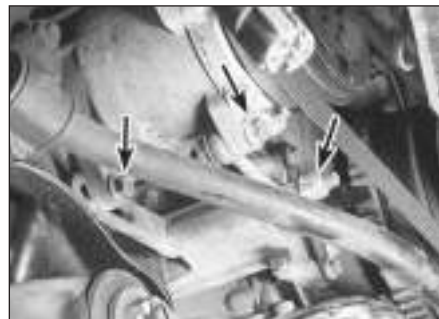
15.5 Remove the lower mounting bolts and the adjuster bolt (arrowed)
