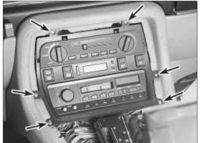
13.3 Remove the retaining screws (arrowed) and pull the radio/control panel out enough to unplug the connectors
