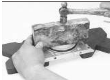
15.4 Drive the new seal into the retainer with a wood block
