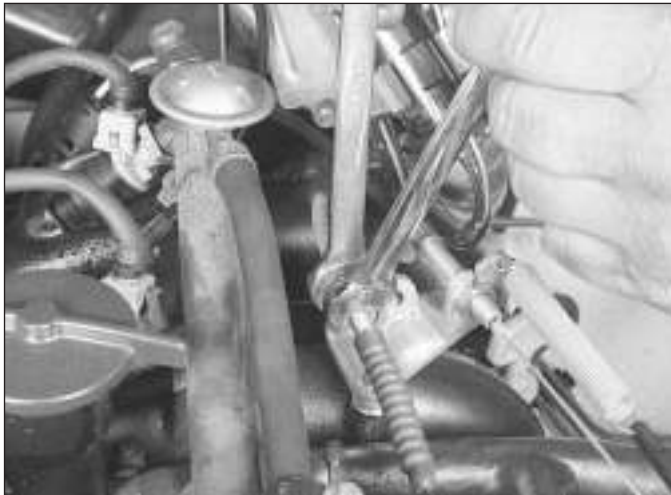
10.2 Loosen the locknuts on the accelerator cable
