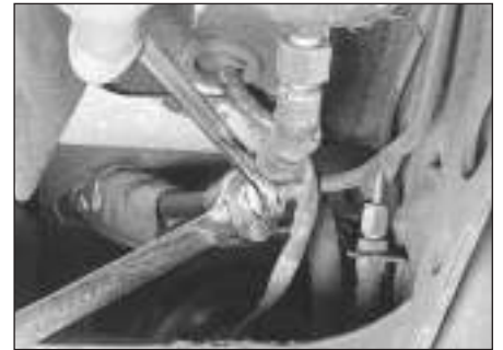
7.9a Disconnect the flexible fuel lines from the metal fuel lines
