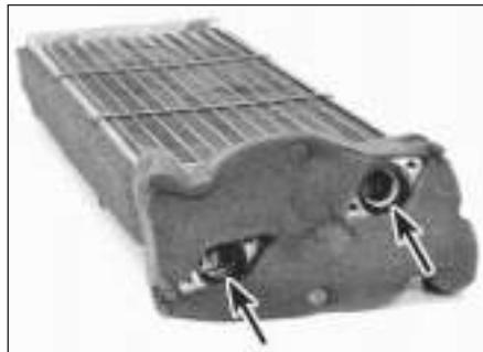
11.9 Retain the original foam insulation on the heater core or transfer to the new core, and replace the two O-rings (arrowed)
