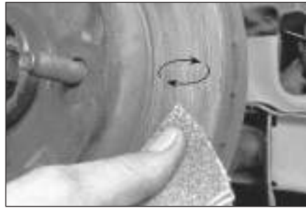
5.4b Using a swirling motion, remove the glaze from the disc surface with sandpaper or emery cloth
