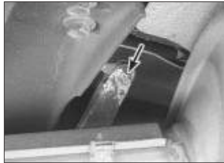
11.3 To disconnect the rear end of the front cable from the adjuster lever, remove this cotter pin, washer and clevis pin (arrowed)
