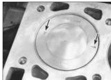
25.9 Pistons must be installed with the arrow (right arrow) or FRONT facing the front of the engine - left arrow indicates piston size letter
