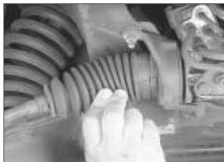
12.8a Check the steering gear dust boots for cracks and leaking steering fluid
