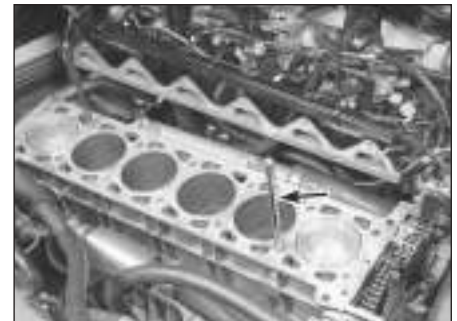
11.20 Fabricate two alignment studs from old cylinder head bolts and refit them in the engine block - after the cylinder head is installed, remove the two studs
