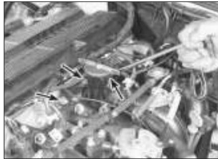
5.6a Remove the oil filler tube bracket nuts (arrowed) . . .
