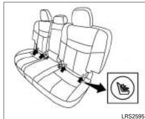
LATCH label locations rear bench
