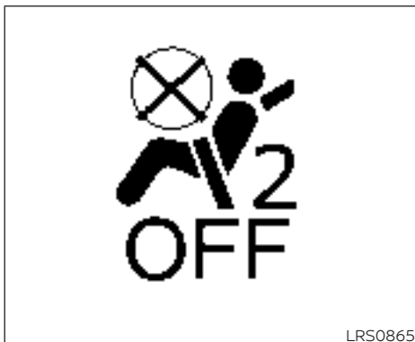
Front passenger air bag and status light
