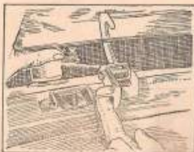
Fig. 9 The bonnet safety catch is released by inserting a finger below the partly raised bonnet and raising the catch lever
