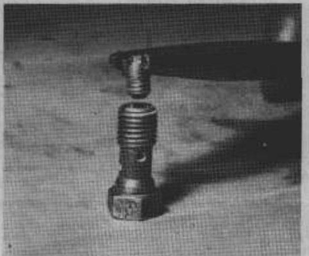
3.6c. If there is dirt behind the jet, take it out of its holder with a screwdriver
