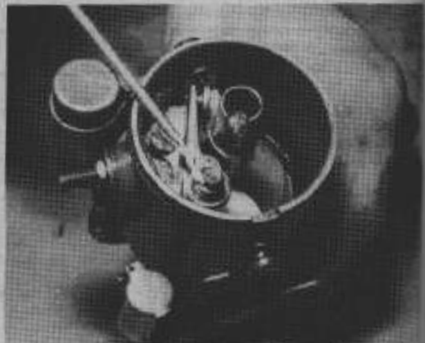
3.6a. Prise off the circlip on the moving contact post. (This distributor has the early type of oiler)
