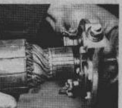
11.1. When it comes to reassembly fit the brush-end to the armature first; so the brushes can be slid easily over the commutator
