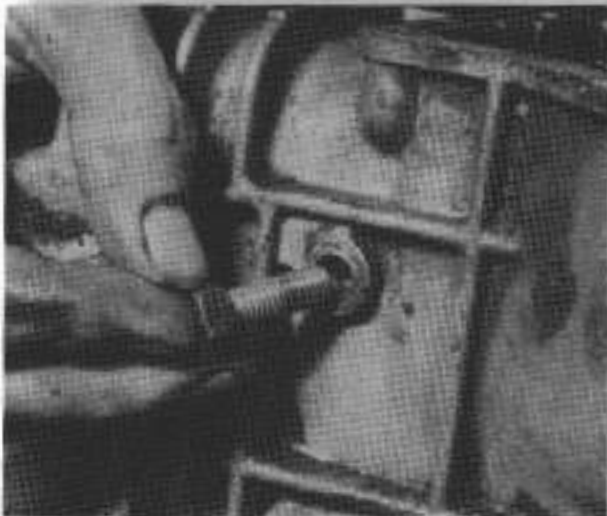
5.13a. The reverse shaft lock-bolt comes out of the casing side
