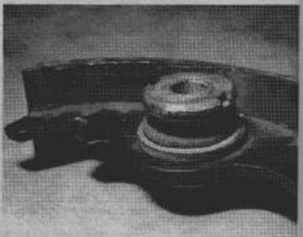
Fig. 7.6. The self adjusters are difficult to undo without special spanners. You can make them out of tubing
