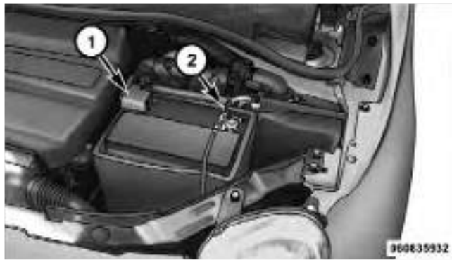
Positive Battery Post
