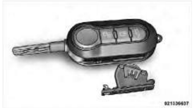
Battery Case Removed
