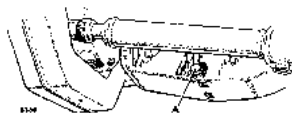
Fig. 9. Engine sump drain plug A—Drain plug
