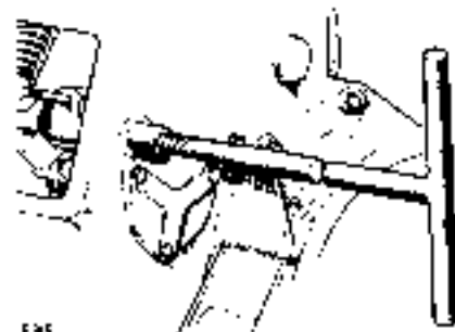
262749. Extractor—side rocker shaft (2.6 Petrol)
