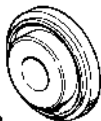
18G 1349. Hub oil seal replacer
