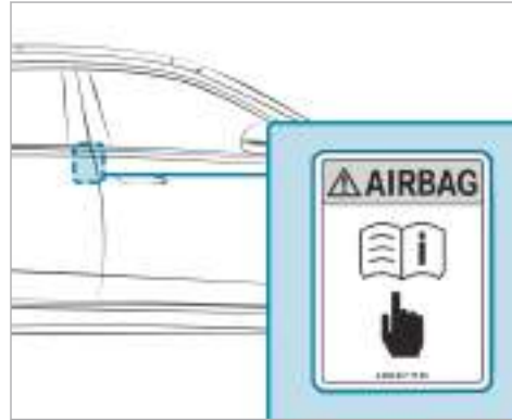
Rear air bag (visible when the left or right rear door is open) (→ page 73)
