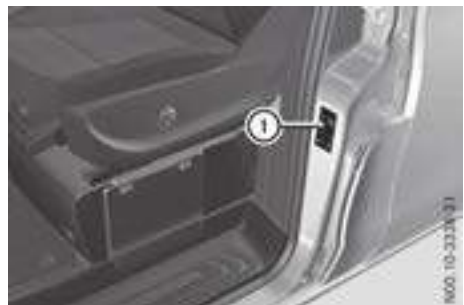
Vehicle identification plate on the driver's side B-pillar
