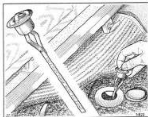
The automatic transmission dipstick markings
